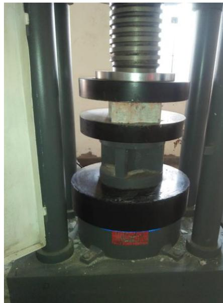
Figure 5. Split Tensile Strength Setup
