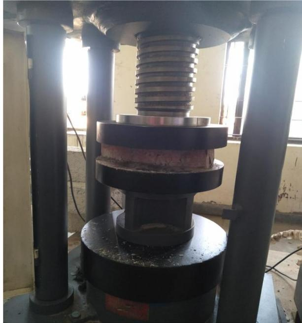
Figure 1. Compression strength test setup
