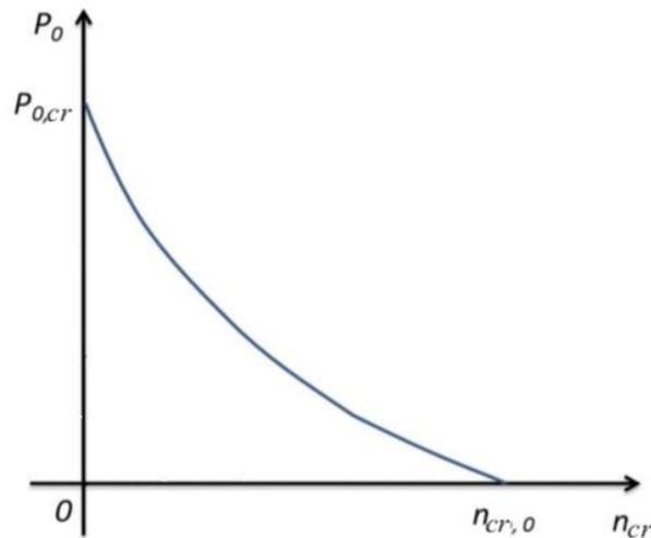
**Fig 2.**The curve of hidden stage of failure in incubation period.
