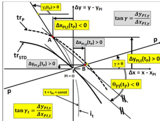
**Fig. 3** The schema for the estimation of non-isochronous perturbations ( $t_{\text{end}} = t_{PI} + \Delta t_{PI,\gamma}$ )  $\Delta x_{PI,\gamma}(t_P)$ ,  $\Delta y_{PI,\gamma}(t_P)$  in the point of impact (burst) PI from the given isochronous perturbations ( $\Delta t_{PI,t} = 0$ )  $\Delta x_{PI,t}(t_P)$ ,  $\Delta y_{PI,t}(t_P)$ .  $tr_{STD}$  – standard trajectory,  $tr_P$  – perturbed trajectory,  $p$  – plane footprint,  $i_t$  – isochrone.
