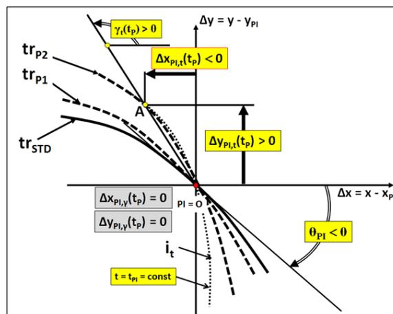
**Fig. 4** The schema for explanation of the exact and strong norm effect problem. It's true for exact norm effect  $\Delta x_{PI,\gamma}(t_p) = 0$  and  $\Delta y_{PI,\gamma}(t_p) = 0$  and for strong norm effect  $\Delta x_{PI,\gamma}(t_p) \approx 0$  and  $\Delta y_{PI,\gamma}(t_p) \approx 0$ ;  $t_p = t_{O,i}$ ,  $tr_{STD}$  – standard trajectory,  $tr_p$  – perturbed trajectory,  $i_t$  – isochrone.
