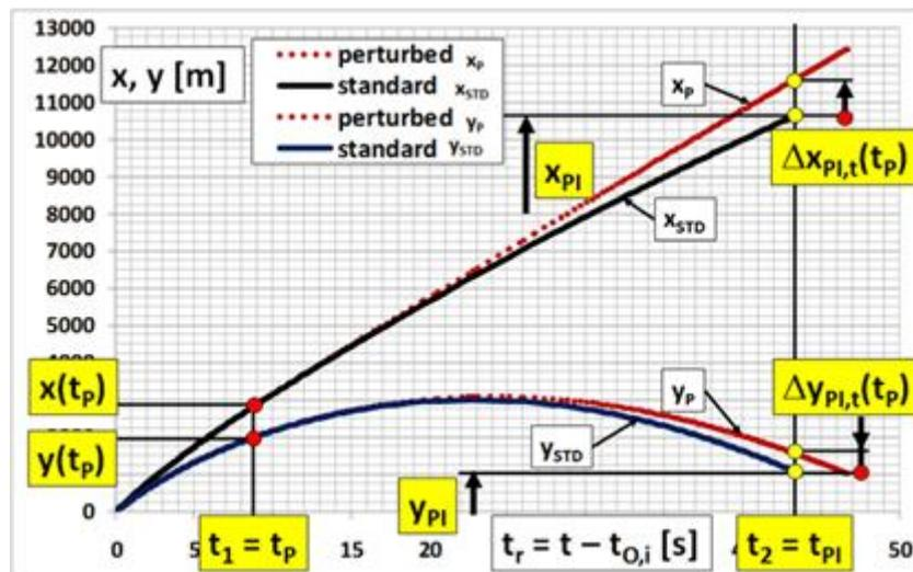
**Fig. 1** Partially perturbed trajectory  $(x_p(t_p), y_p(t_p))$  and its isochronous perturbations ( $\Delta t_{PI} = 0$ )  $\Delta x_{PI,t}(t_p)$ ,  $\Delta y_{PI,t}(t_p)$  in the point of impact (burst) PI  $(x(t_{PI}), y(t_{PI}))_{STD} = (x_{PI}, y_{PI})_{STD}$ .
