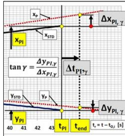
Fig. 2 Zoom of the Fig. 1 and non-isochronous perturbations ( $t_{end} = t_{PI} + \Delta t_{PI,\gamma}$ )  $\Delta x_{PI,\gamma}(t_P)$ ,  $\Delta y_{PI,\gamma}(t_P)$  in the point of impact (burst) PI.
