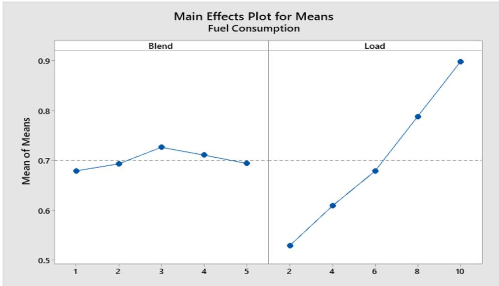
Figure 8: Main Effects Plot for Means of Fuel Consumption
