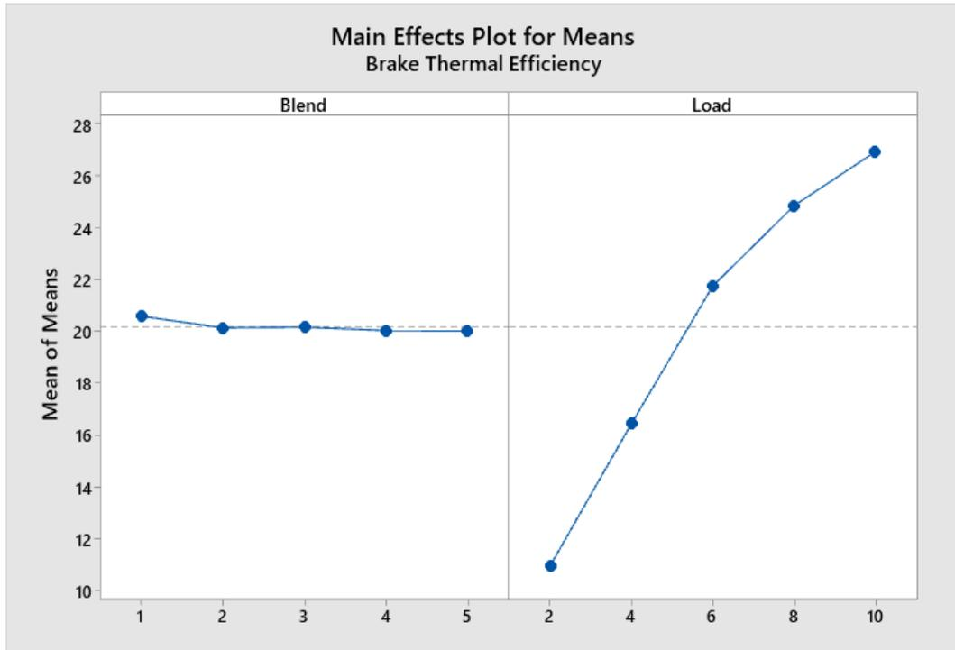
Figure 4: Main Effects Plot for Means of Brake Thermal Efficiency
