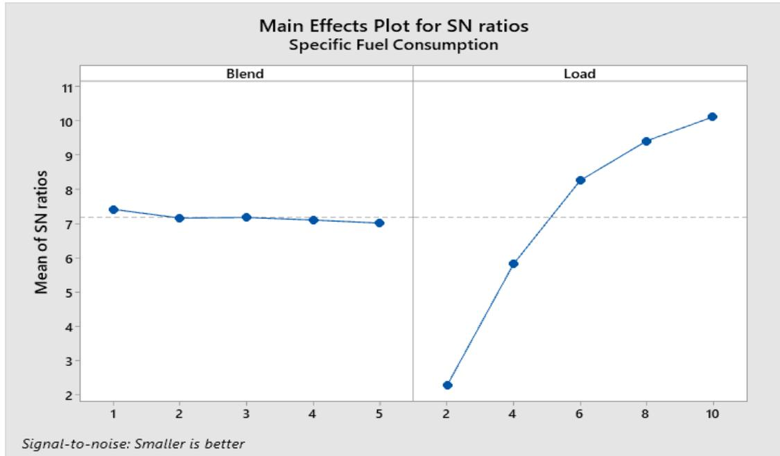
Figure 7: Main Effects Plot For S/N Ratio of Specific Fuel Consumption
