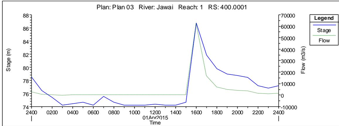
**Figure 5.4 (a):** Stage and flow hydrographs for river station 400
