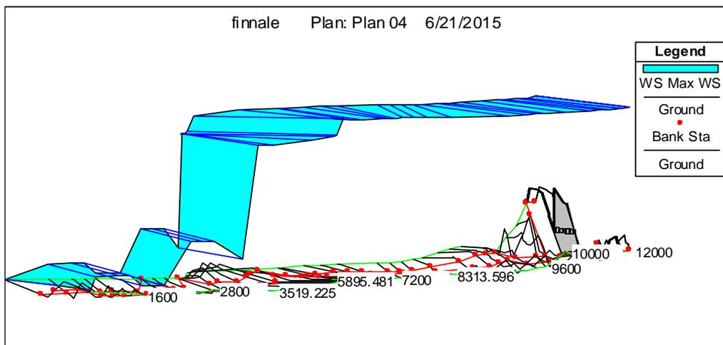
Figure 5.7: 3-D view of water surface elevation of Jawai downstream
