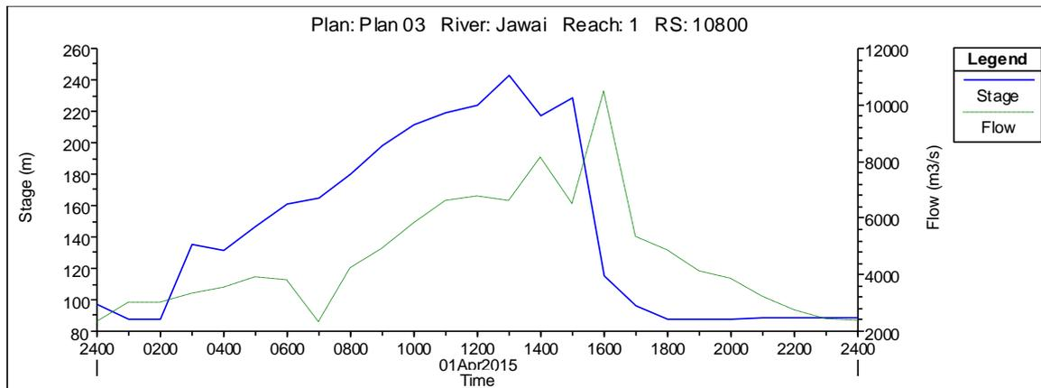
**Figure 5.3 (a): Stage and flow hydrographs for river station 10800**
