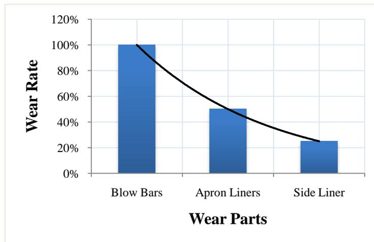
**Figure 3** Wear comparisons of an impact wear parts [5].
