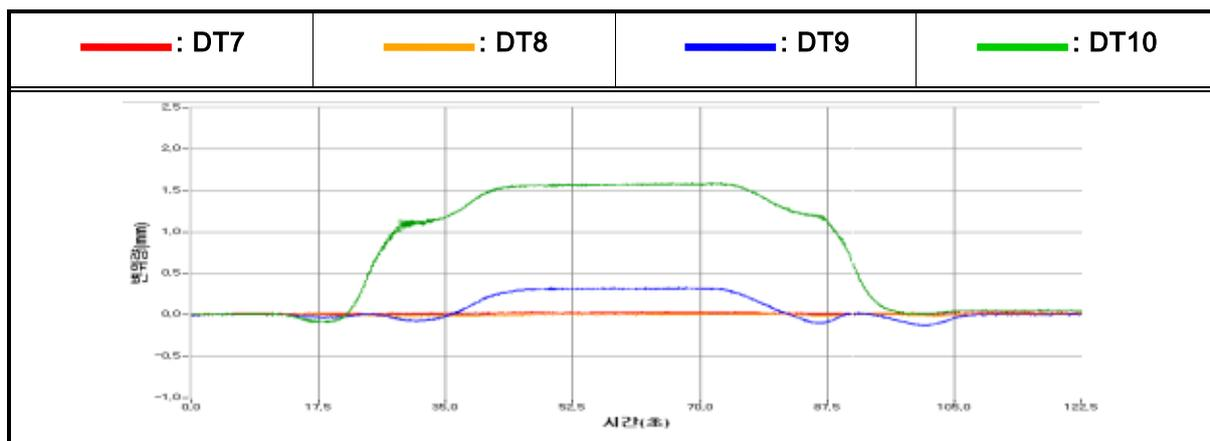
Fig no 3-f. Variation of displacement with time (section C-C : DT7, DT8, DT9, DT10) - LC8
