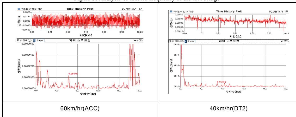
Fig no 6. FFT Analysis result for acceleration response curve
