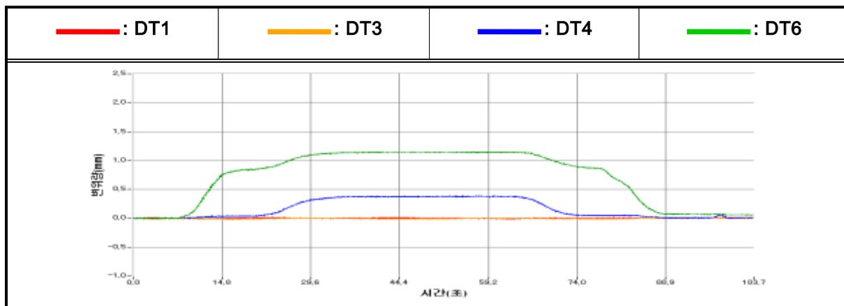
Fig no 3-d. Variation of displacement with time (section A-A : DT1, DT3, DT4, DT6) - LC4
