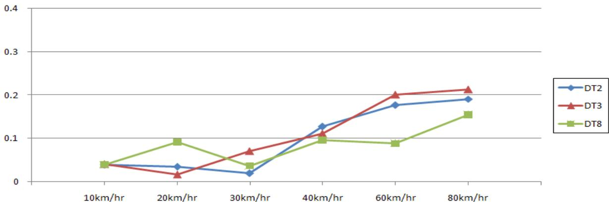
Fig no 4. Variation of impact factor with vehicle’s velocity
