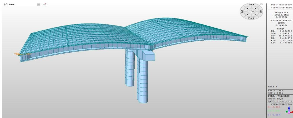
Fig no 5. Analysis of natural frequency of the test bridge
