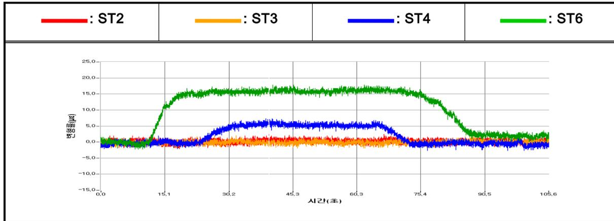
Fig no 3-b. Variation of strain with time (section A-A : ST2, ST3, ST4, ST6) - LC4
