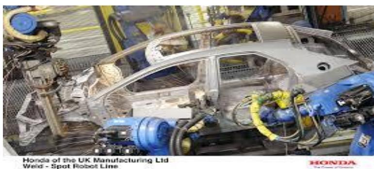
*Figure12: Honda Weld - Spot Robot Line*
