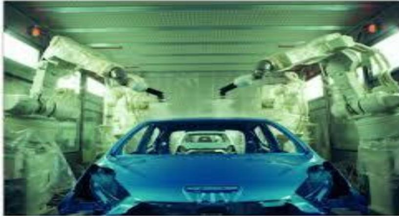
**Figure 1:** Robotics application in automotive painting
