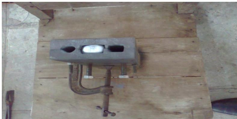
**Fig.2.1.2 Metal Die (CI) with proper fixtures.**
