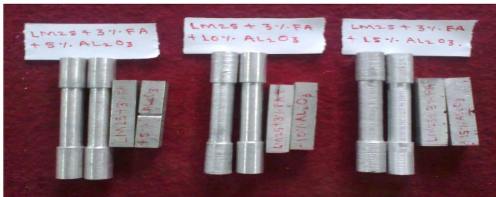
**Fig 2.1.5 Tensile and impact test specimen with varying composition of Al<sub>2</sub>O<sub>3</sub>**
