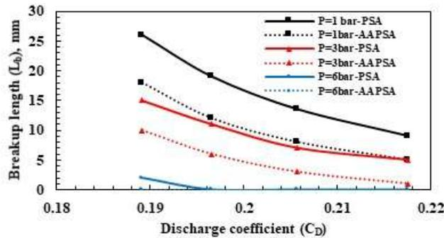
Fig. 5 Effect of discharge coefficient on the breakup length at different injection pressures [ $D_o/L_o=0.27$ ,  $W \times H=1.5 \times 1.5$  and  $\theta = 90^\circ$ ]
