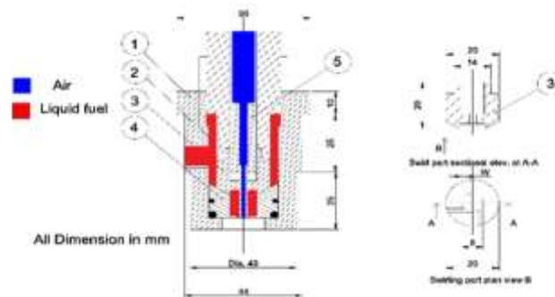
**Fig. 2** Detailed dimensions of the air assisted pressure swirl atomizer
