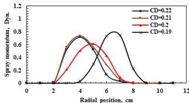
Fig. 10 Radial distribution of calculated spray momentum at different values of  $C_D$  of AAPSA with 2 g/s [P = 9 bar,  $W \times H = 1.5 \times 1.5$  and  $L/D_o = 0.25$ ]
