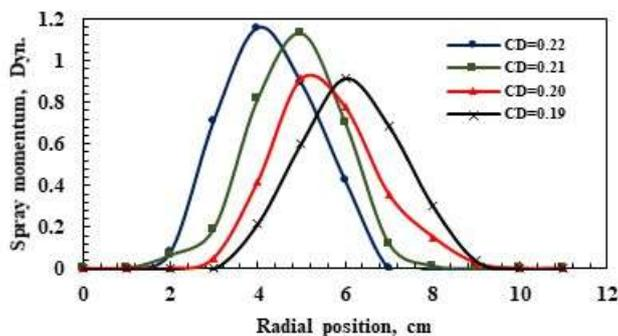
**Fig. 11** Radial distribution of measured spray momentum at different values of  $C_D$  of AAPSA with 2 g/s [ $P = 9$  bar,  $W \times H = 1.5 \times 1.5$  and  $L/D_o = 0.25$ ]
