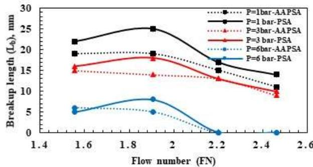
Fig. 4 Effect of flow number on the breakup length at different injection pressures [ $D_o/L_o=0.27$ ,  $L_s/D_s=0.93$  and  $\theta = 90^\circ$ ]
