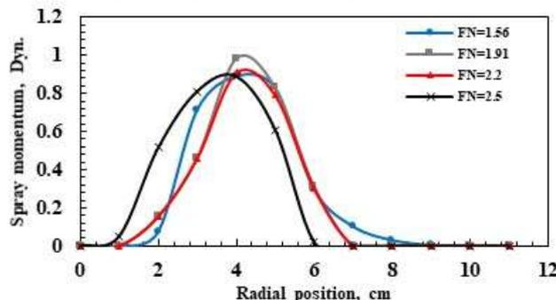
**Fig. 8** Radial distribution of measured spray momentum at different values of FN of AAPSA with 2 g/s [P = 4 bar,  $L_s/D_s = 0.775$  and  $L/D_o = 0.25$ ]
