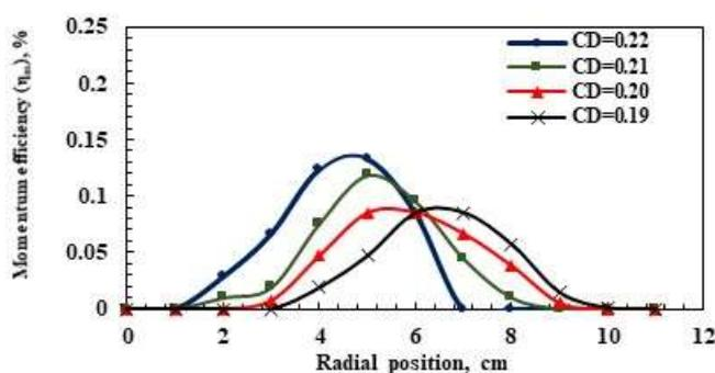
**Fig. 12** Radial distribution of momentum efficiency at different values of  $C_D$  of AAPSA with 2 g/s [ $P = 9$  bar,  $W \times H = 1.5 \times 1.5$  and  $L/D_o = 0.25$ ]
