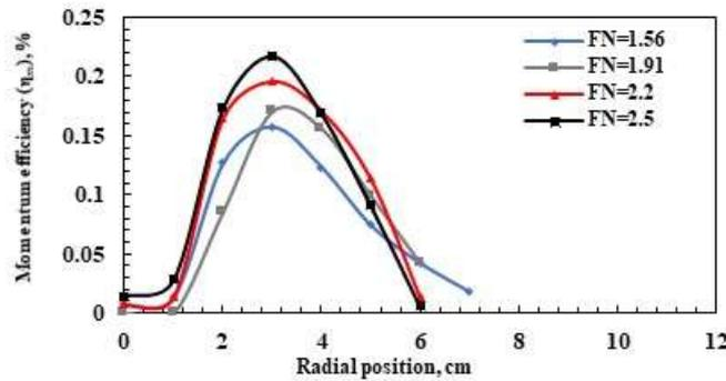
Fig. 9 Radial distribution of spray momentum efficiency at different values of FN of AAPSA with 2 g/s [P = 4 bar,  $L_s/D_s = 0.775$  and  $L/D_o = 0.25$ ]
