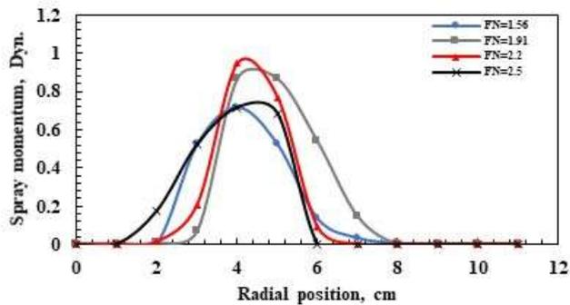
**Fig. 7** Radial distribution of calculated spray momentum at different values of FN of AAPSA with of 2 g/s [P = 4 bar,  $L_s/D_s = 0.775$  and  $L/D_o = 0.25$ ]
