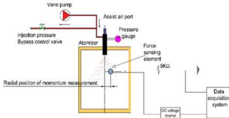
**Fig. 1** Schematic diagram of momentum the test rig
