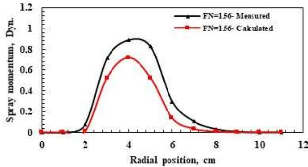
**Fig. 6** Radial distribution of measured and calculated spray momentums of AAPSA with 2 g/s [P = 4 bar,  $L_s/D_s = 0.775$ , FN=1.56 and  $L/D_o = 0.25$ ]
