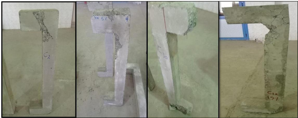
Fig. (19):mode failure of the tested columns of group B
