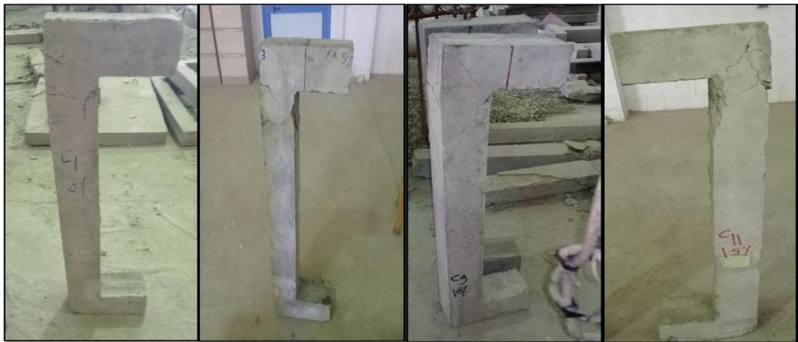
Fig. (16):Mode Failure Of The Tested Columns Of Group A
