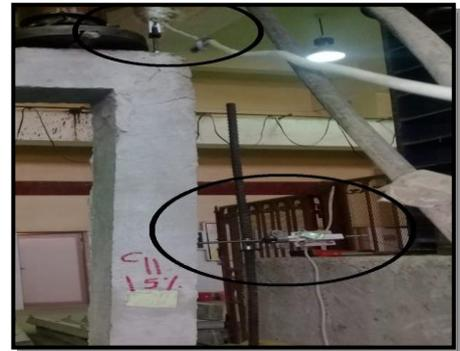
Fig.(13): LVDT Used in Lap
