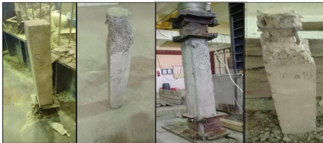
Fig. (19): Mode Failure Of The Tested Columns Of Group C
