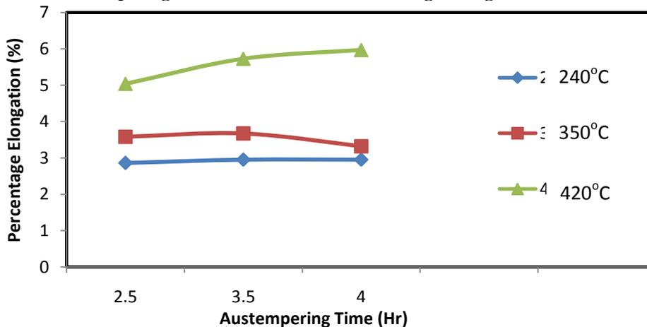
Fig. 3.2: Effect of austempering temperature and time on the percentage elongation of ADI material
