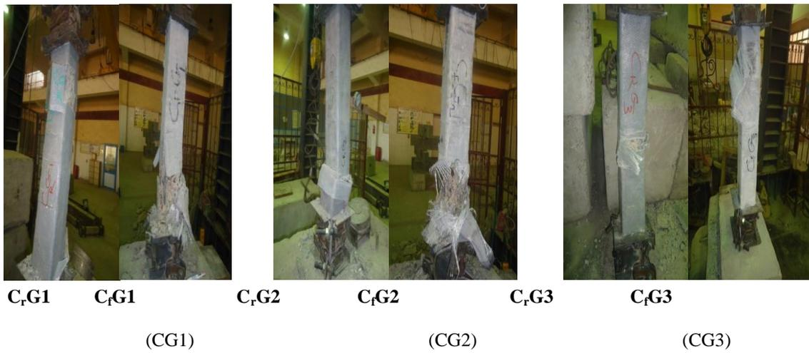
**Fig. 12** failure mode for series (CG) before and after fire exposure
