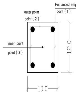
**Fig.10:** The furnace with column model and thermal measuring points
