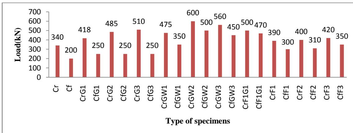
**Fig.4:** Ultimate load for all specimens.
