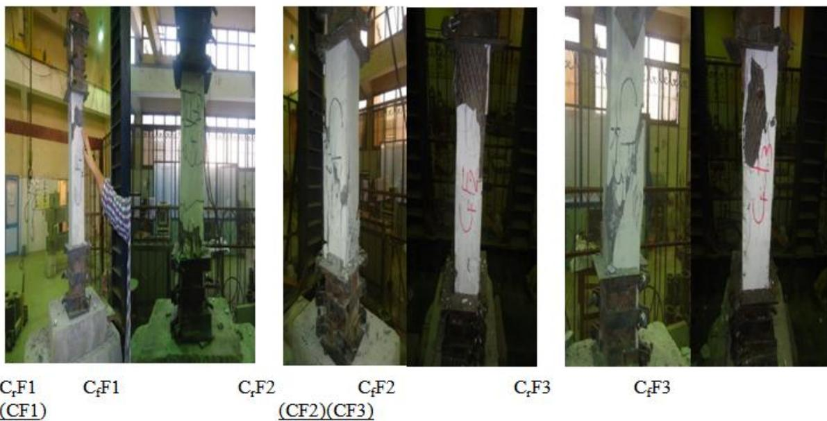
**Fig. 14** failure mode for series (CF) before and after fire exposure
