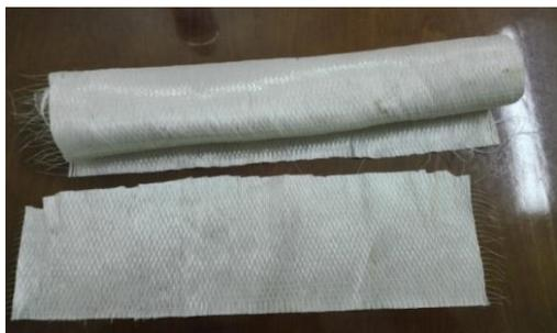
**Fig.1** GFRP Laminate (Sikawrap)
