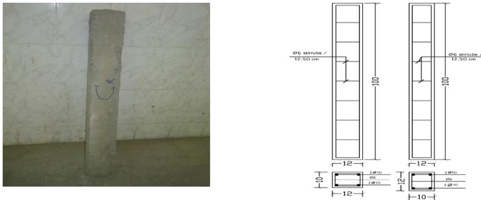
Fig. 3 Cross section of the control columns
