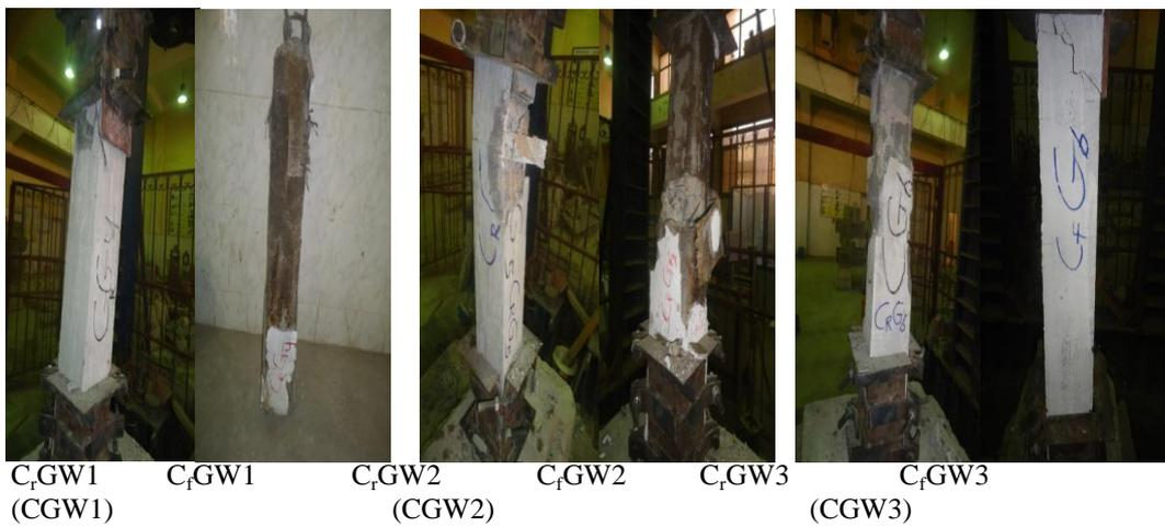
**Fig. 13** failure mode for series (CGW) before and after fire exposure
