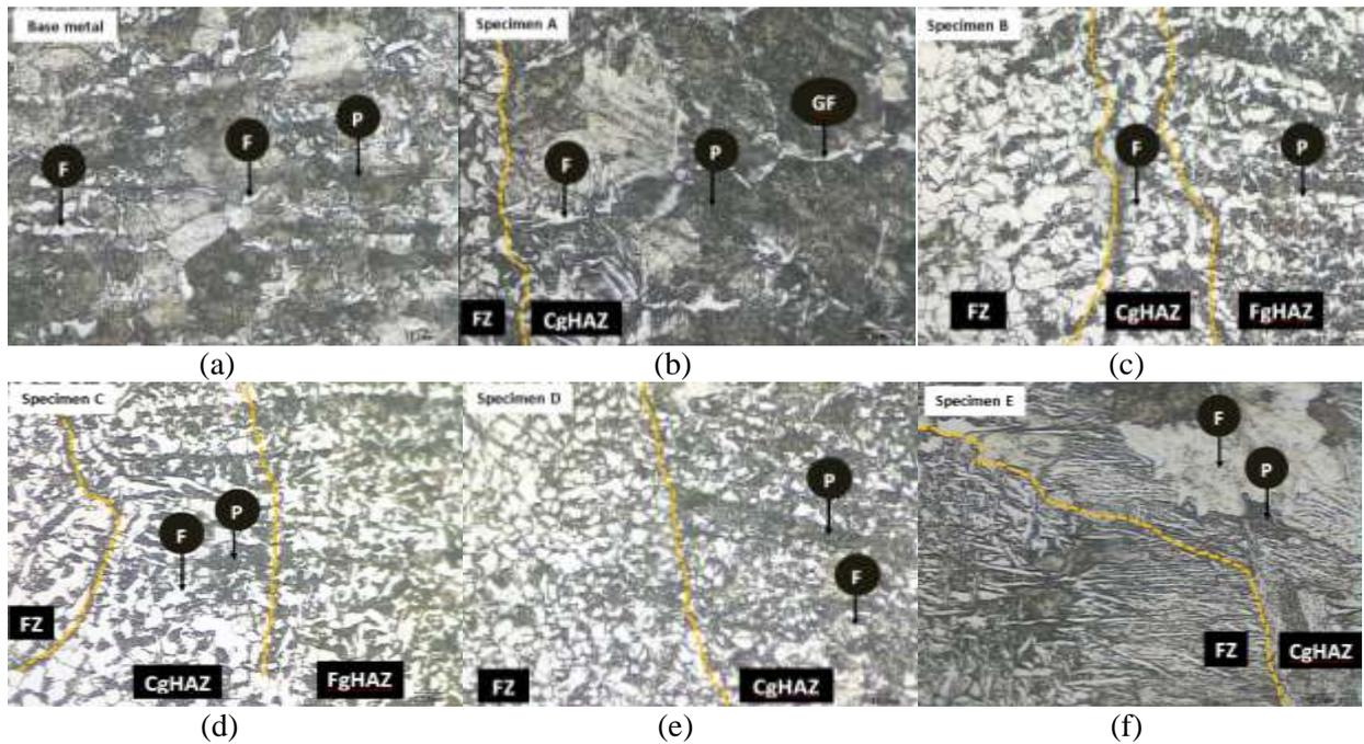
**Figure 3.**HAZ microstructure at 500 times magnification for (a) Base metal, (b) Specimen A, (c) Specimen B, (d) Specimen C, (e) Specimen D, (f) Specimen E. F for Ferrite, P for Pearlite, GF for grain boundary Ferrite, FZ for Fusion Zone, FgHAZ for Fine grain HAZ and CgHAZ for Coarse grain HAZ
