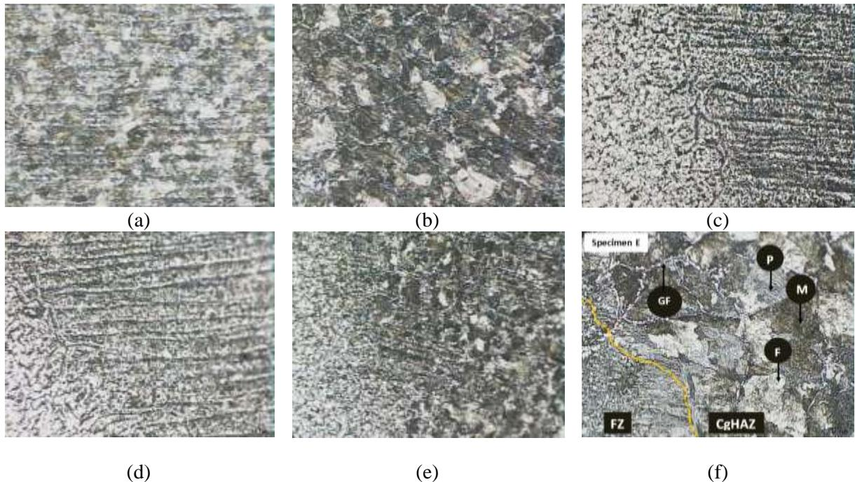
**Figure 4.**HAZ microstructure at 200 times magnification for (a) Base metal, (b) Specimen A, (c) Specimen B, (d) Specimen C, (e) Specimen D, (f) Specimen E. M for Martensite
