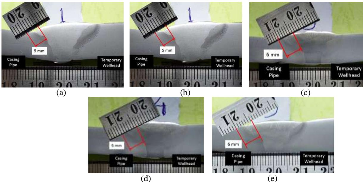
**Figure 2.**HAZ of the cross section of (a) Specimen A, (b) Specimen B, (c) Specimen C, have the same width, 5 mm. And (d) Specimen D, (e) Specimen E have the same width are 6 mm
