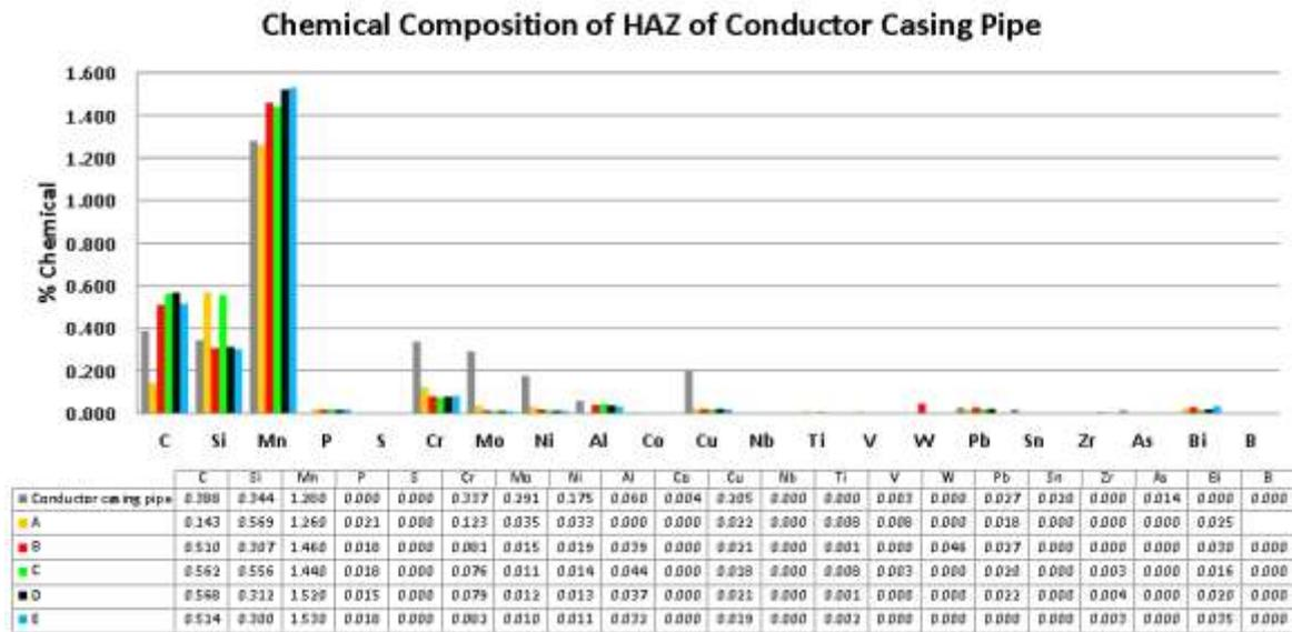
Figure 5. Chemical composition in HAZ of each specimen of Conductor Casing Pipe
