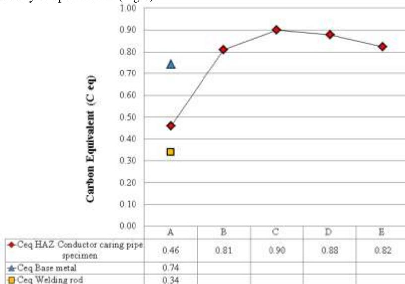
Figure 6. Trend of Ceq of Conductor Casing Pipe as function of repeated welding of Temporary Wellhead
