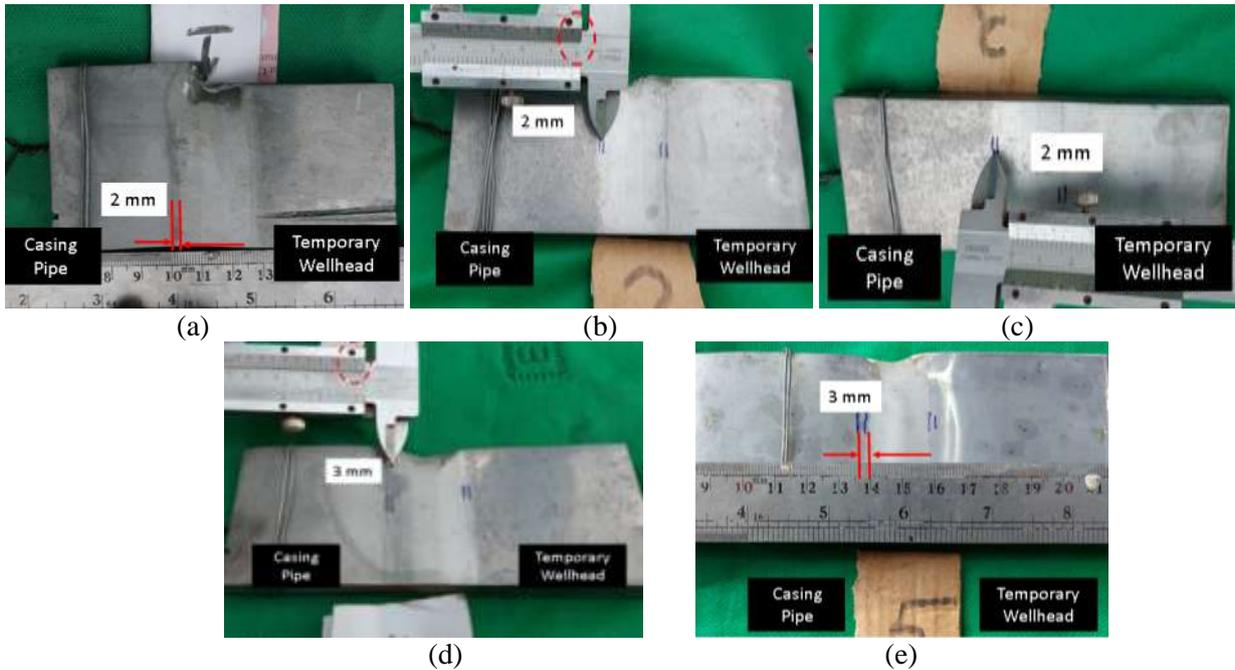
**Figure 1.**HAZ of the outer surface of (a) Specimen A, (b) Specimen B, (c) Specimen C, have the same width, 2 mm. And (d) Specimen D, (e) Specimen E have the same width are 3 mm
