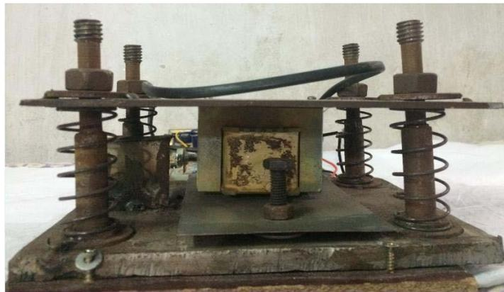
Fig.3: Model structure of vibration control system
