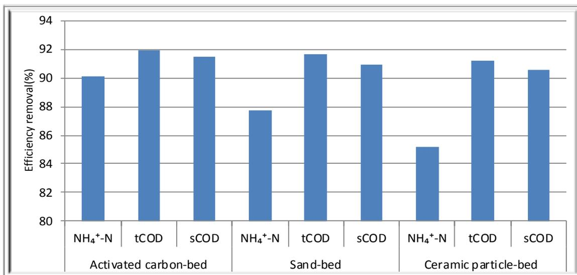
Figure no. 6: The average efficiency removal of tCOD, sCOD, and  $\text{NH}_4^+$ -N comparison.
