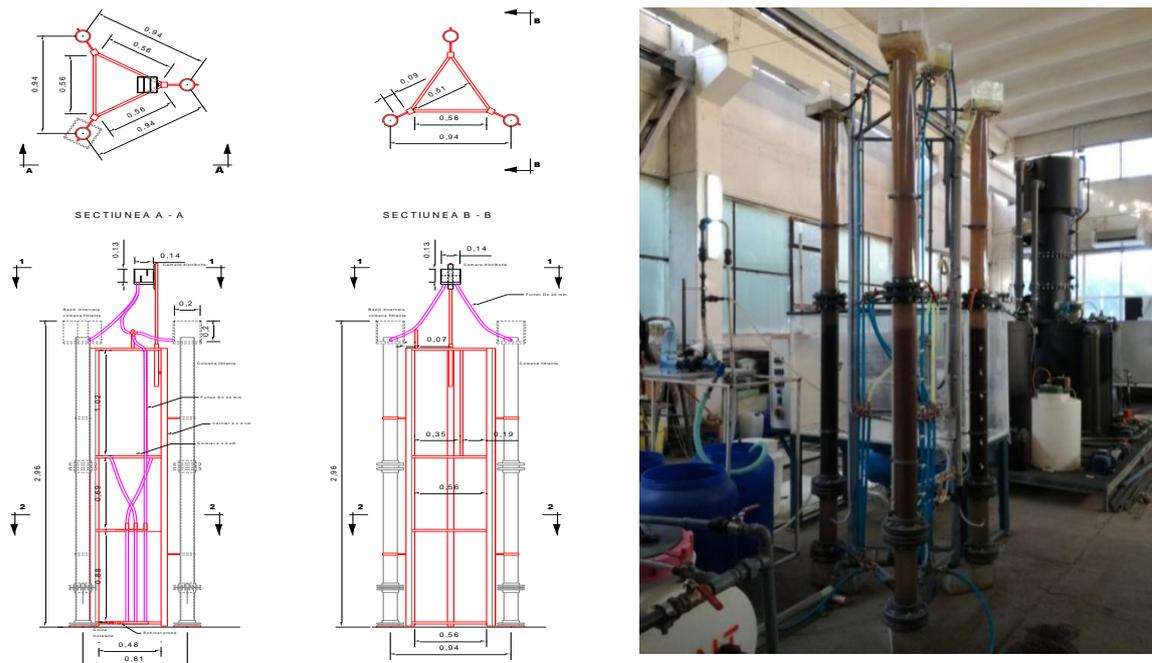
**Figure no. 1:** Schematic diagram and Photograph of the pilot scales of BAF
