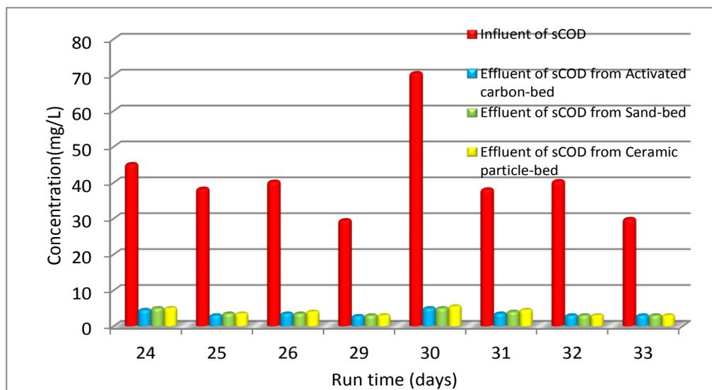
**Figure no. 4:** The influent and effluent concentration of sCOD comparison.
