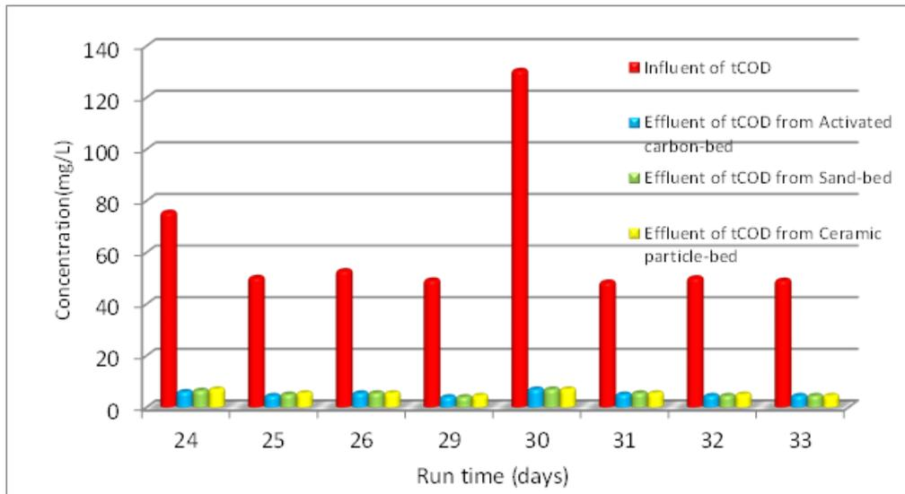
**Figure no. 3:** The influent and effluent concentration of tCOD comparison.
