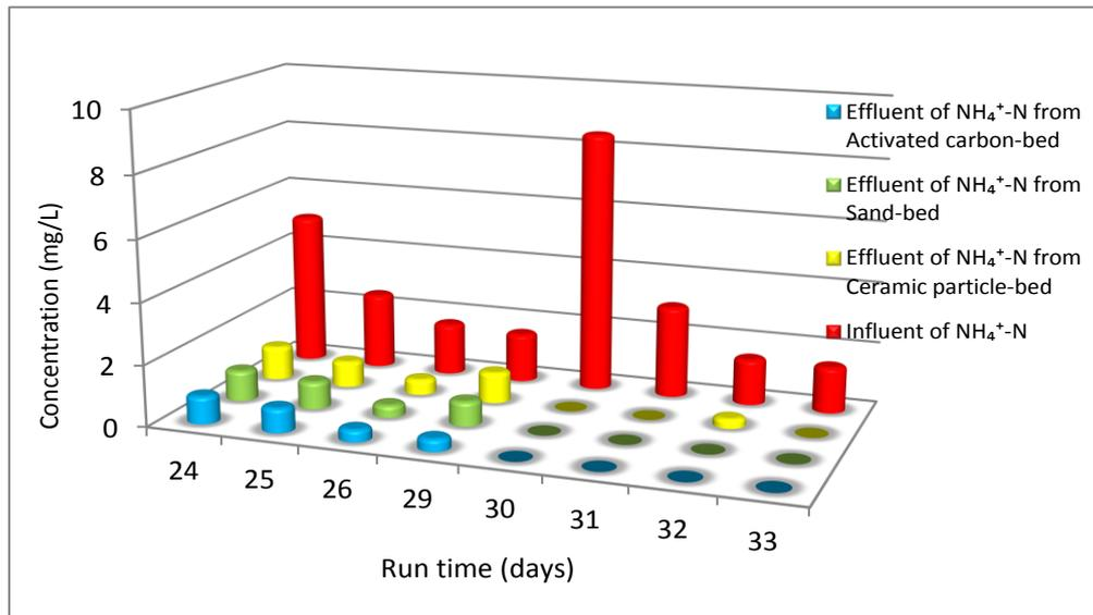
Figure no. 5: The influent and effluent concentration of  $\text{NH}_4^+$  comparison.
