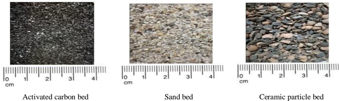
**Figure no. 2:** View of filtration media-based beds used in the pilot scales of BAF.
