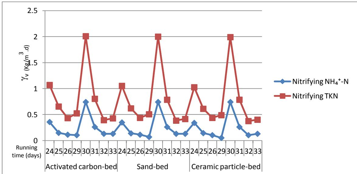
**Figure no. 7:** Mass removal of NH<sub>4</sub><sup>+</sup> and TKN comparison.
