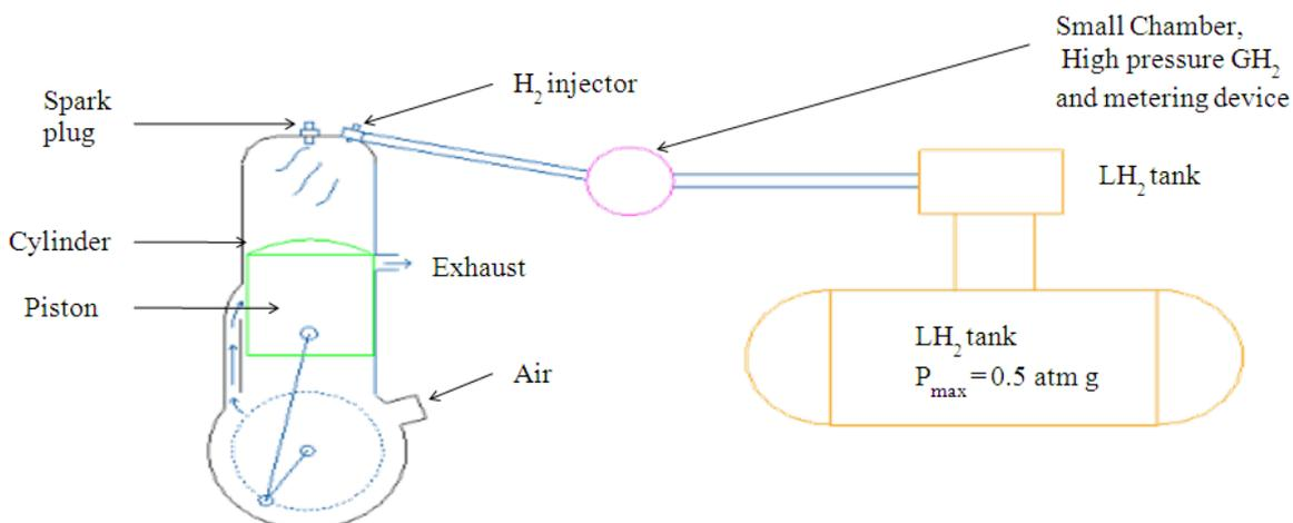
Figure no 1: Liquid hydrogen storage and gaseous hydrogen injection
