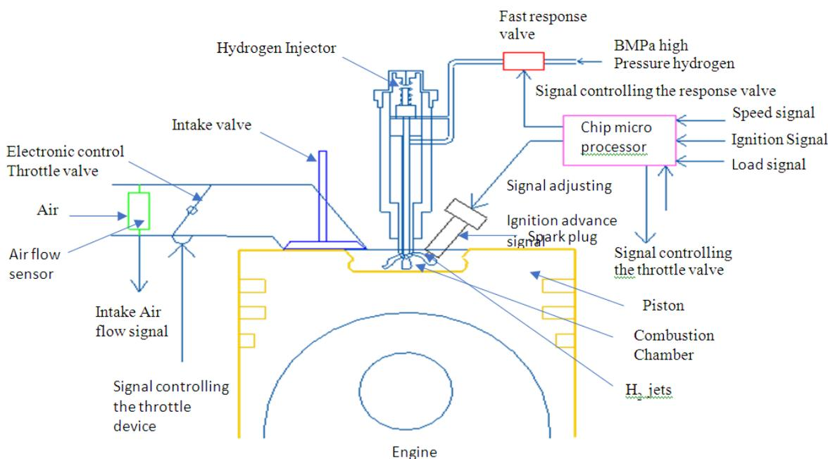
Figure no 2: Hydrogen induction in spark ignition engine
