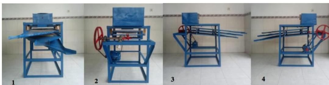
Figure 3.2 The Results of Rice Sorting Machine Design (1. Back View, 2. Front View, 3. Right Side View, and 4. Left Side View)
