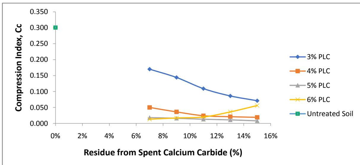
Figure 3: Compression Index,  $C_c$  of PLC and RSCC Modified Cohesive Soil
