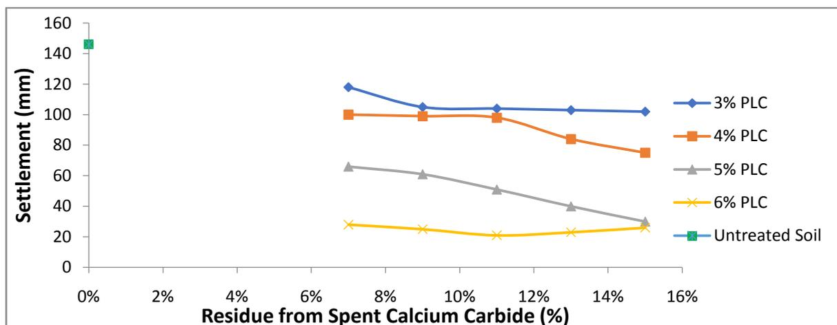
Figure 5: Settlement of PLC and RSCC Modified Cohesive Soil
