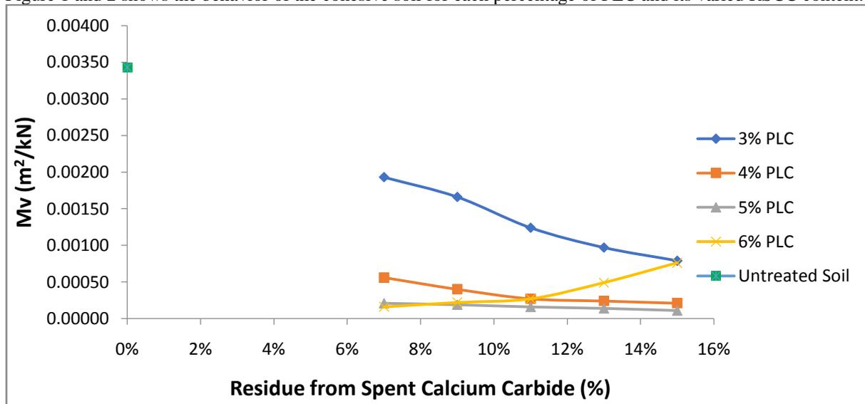
**Figure 1: Coefficient of Volume Change,  $m_v$  of PLC and RSCC Modified Cohesive Soil**
