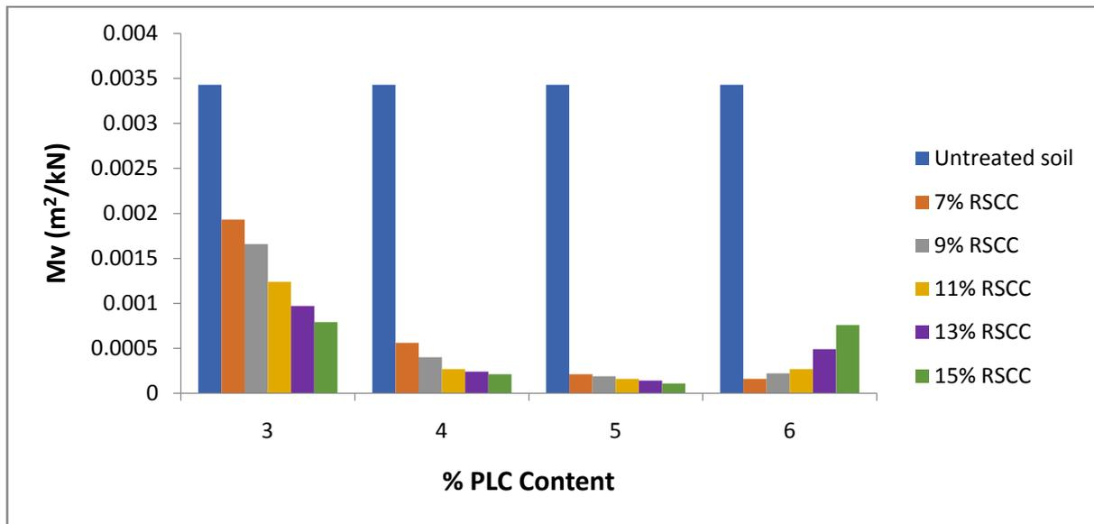
Figure 2: Bar Chart Showing  $m_v$  of PLC and RSCC Modified Cohesive Soil
