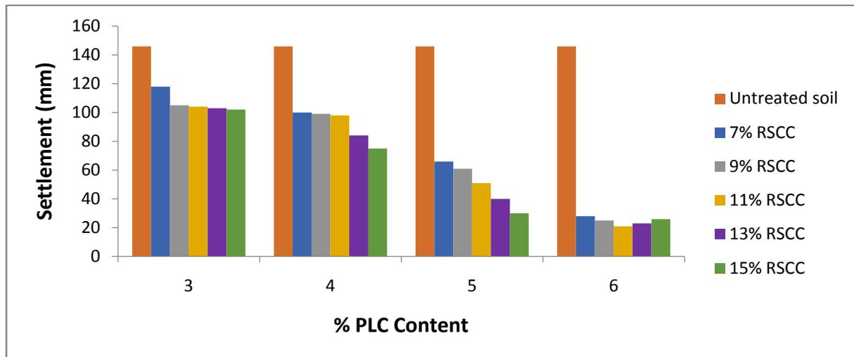
Figure 6: Bar Chart Showing Settlement of PLC and RSCC Modified Cohesive Soil
