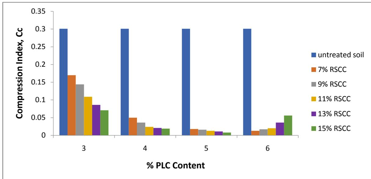
Figure 4: Bar Chart Showing  $C_c$  of PLC and RSCC Modified Cohesive Soil
