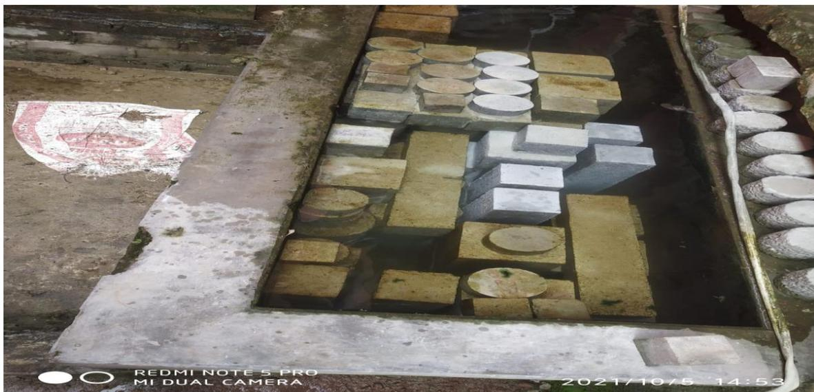
Figure 2 photographic view of cylindrical samples
