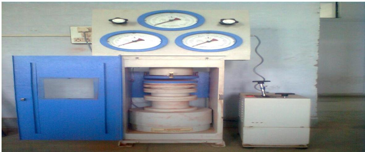
Figure 1 Compressive Strength Testing Machine
