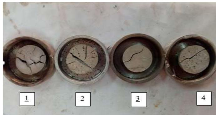
**Fig. 14** Shows the shape of the cracks by shrinkage limit test
