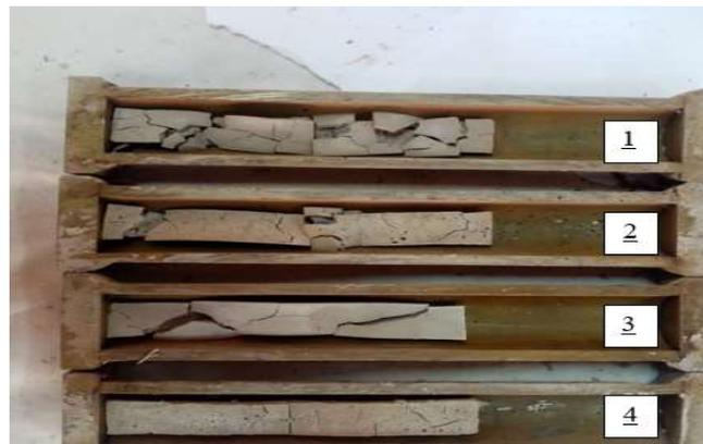
**Figure 15** shows the shape of the cracks by a linear shrinkage test.
