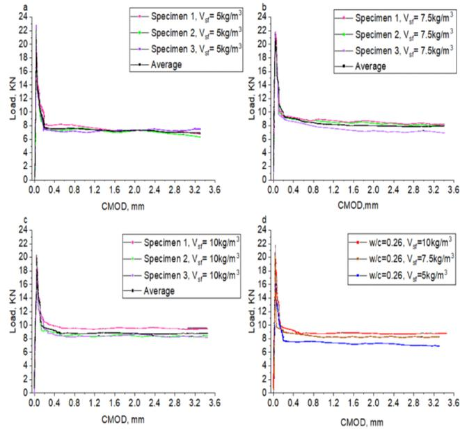
Fig. 2: Load-CMOD for concrete members with different dosages of synthetic fibres
