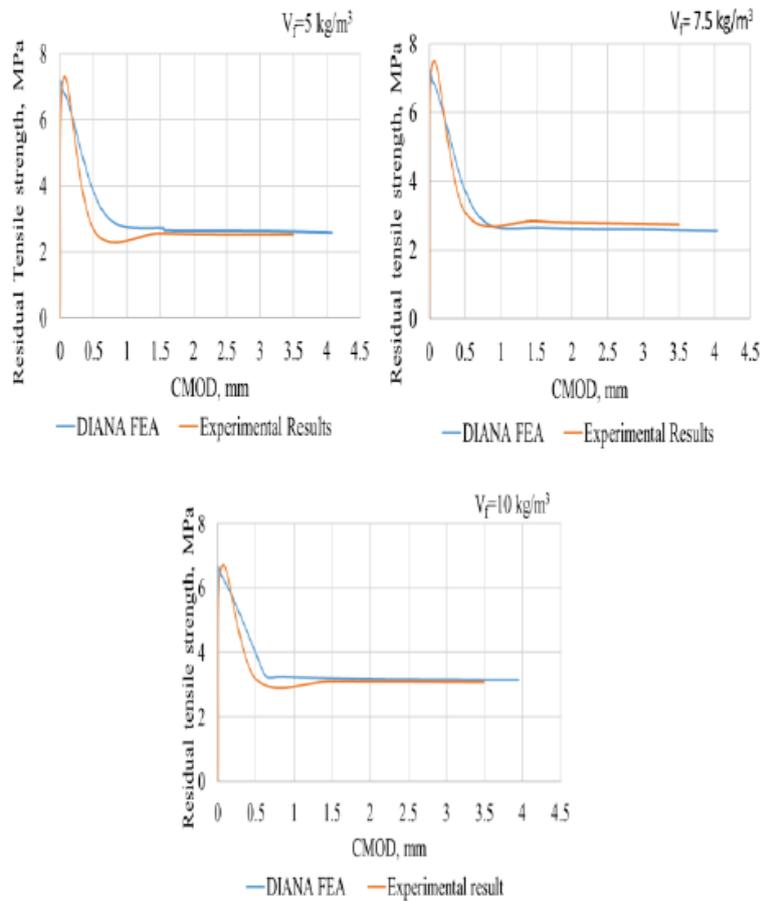
**Fig. 4:** Comparison between residual tensile strength-CMOD curves obtained experimentally and in DIANA FEA
