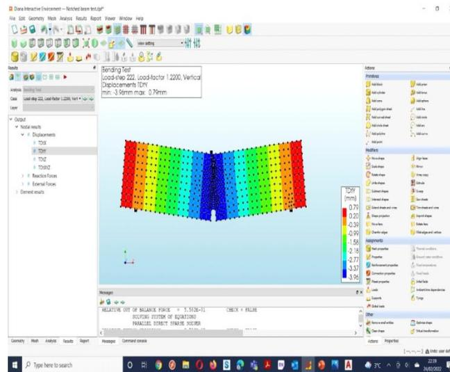
Fig. 3: Vertical displacement obtained from DIANA
