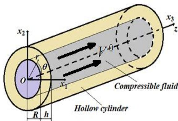
Fig. 1 The sketch of the hydro-elastic system under consideration: (a) cylinder containing flowing fluid; (b) initial pressure and density of the fluid.
