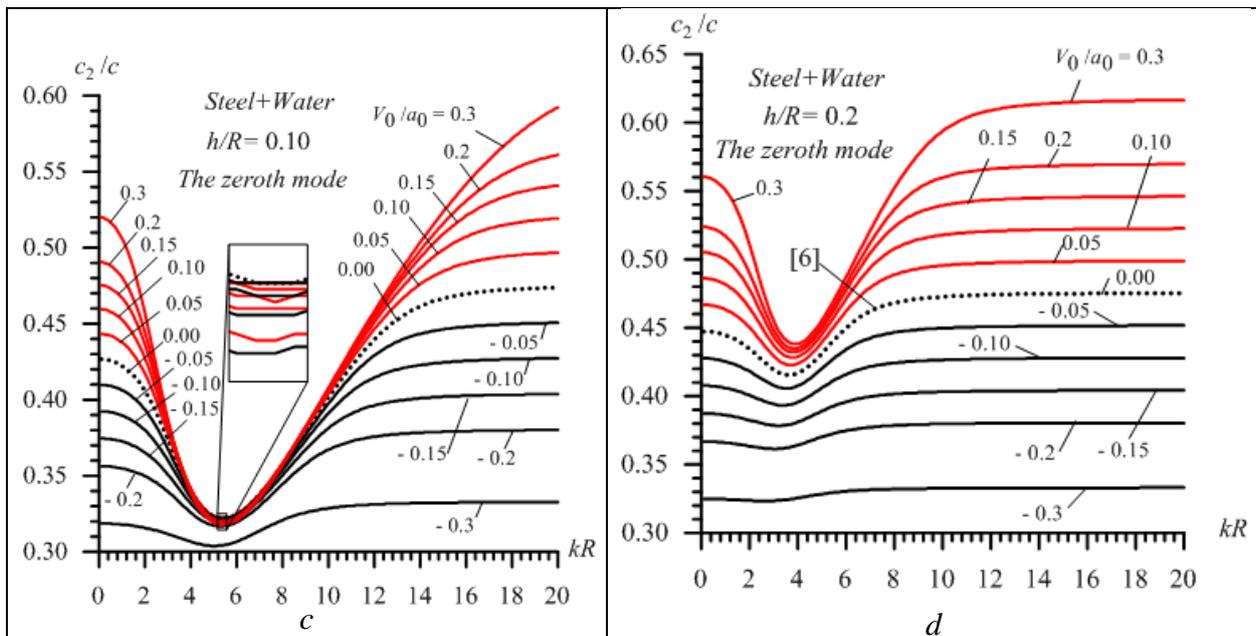
Fig. 2. The influence of the fluid flow velocity and direction on the propagation velocity of axisymmetric longitudinal quasi-Scholte waves propagating in a hollow cylinder containing this fluid in the cases  $h/R=0.03$  (a);  $0.05$  (b);  $0.10$  (c) and  $0.20$  (d)
