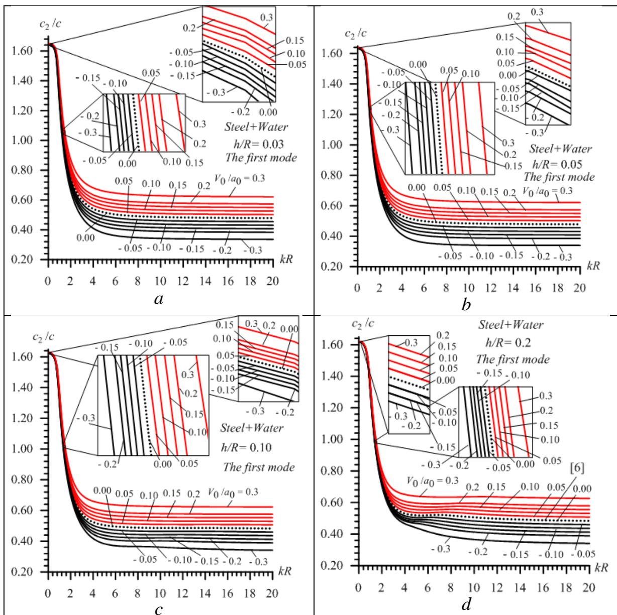
Fig. 3. The influence of the fluid flow velocity and direction on the propagation velocity of axisymmetric longitudinal waves for the first mode propagating in a hollow cylinder with this fluid in the cases  $h/R=0.03$  (a);  $0.05$  (b);  $0.10$  (c) and  $0.20$  (d)
