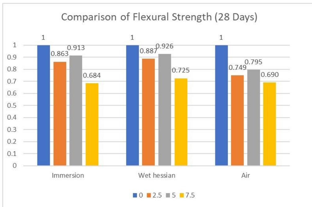
Figure 8. Comparison of the flexural strength of green concrete with normal concrete at the age of 28 days
