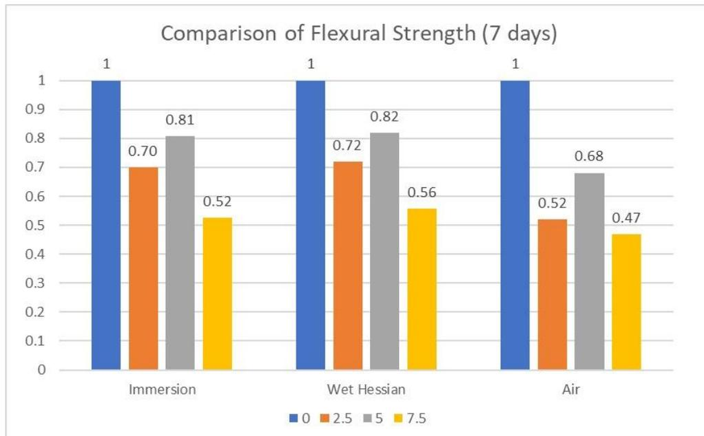
Figure 7. Comparison of the flexural strength of green concrete with normal concrete at the age of seven days
