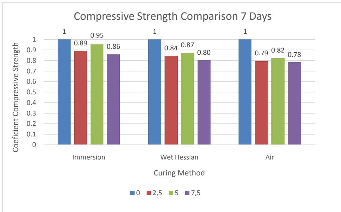
Fig 5 The comparison of the compressive strength of the test object to the control test object at the age of 7 days.
