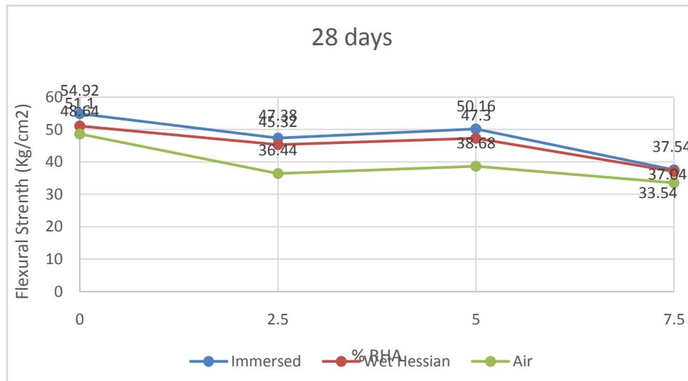
Figure 4. Flexural Strength Test Results of Concrete at 28 days of age
