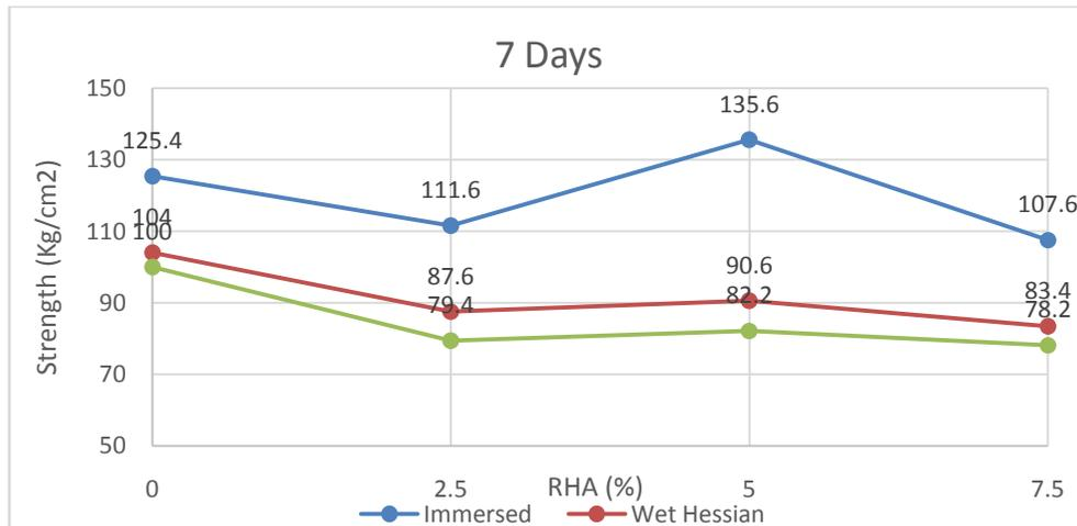
Figure 1. The Concrete Compressive Strength Test at age 7
