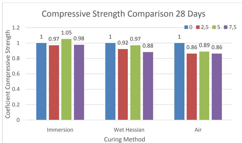
Fig 6 The comparison of the compressive strength of the test object to the control test object at the age of 28 Days
