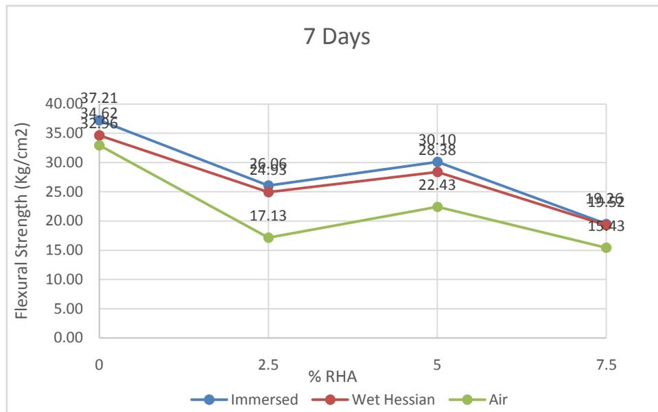
Figure 3. Flexural Strength Test Results of Concrete at the age of 7 days
