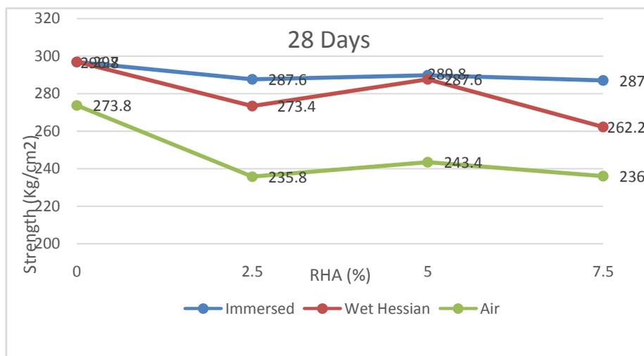
Figure 2. Results of Concrete Compressive Strength Test at 28 days of age
