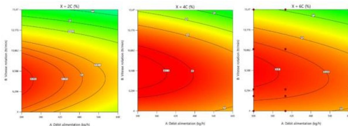
Figure 8: Efficiency as function of rotational speed and flow rate
