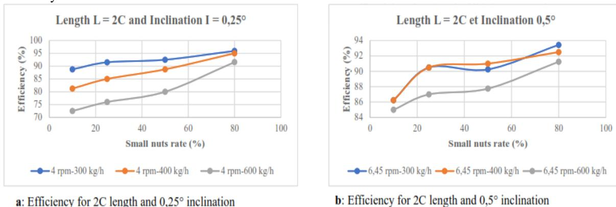
**Figure 3:** Efficiency of calibrator for a short drum
