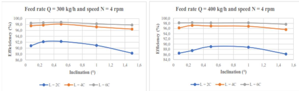
**a:** Efficiency at (300 kg/h; 4 rpm)
