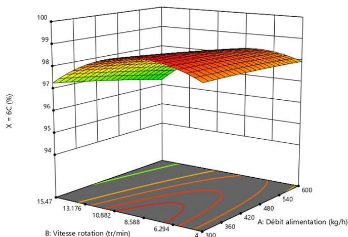
Figure 11: Response surface for a 6C long drum at 0.25° inclination
