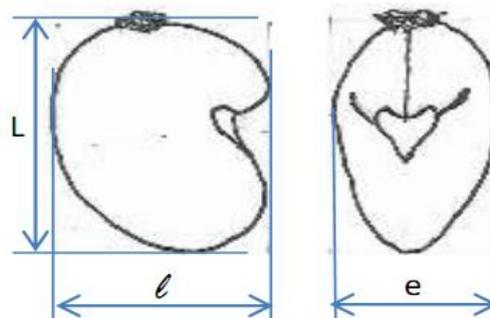
**Figure 1:** Main dimensions of a cashew raw nut: L = Length;  $l$  = width; e = thickness
