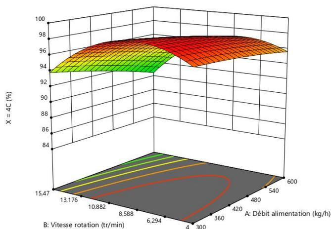
Figure 10: Response surface for a 4C long drum at 0.25° inclination
