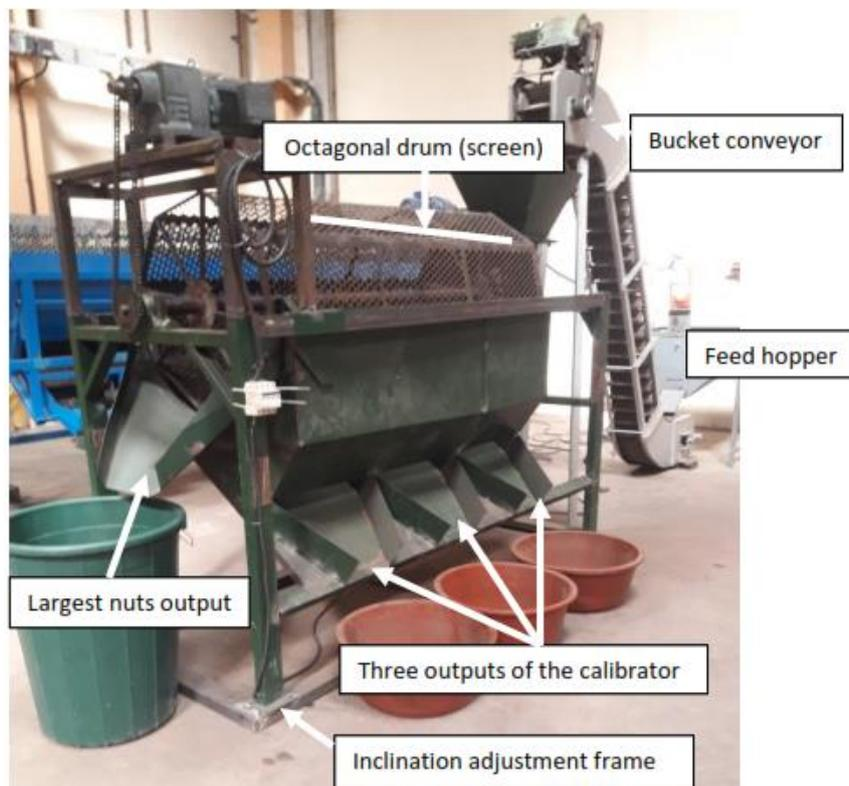
Figure 2: Pilot calibrator of raw cashew nuts.
