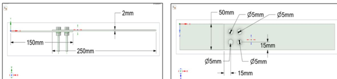
Figure 1: Geometry of the Beam
