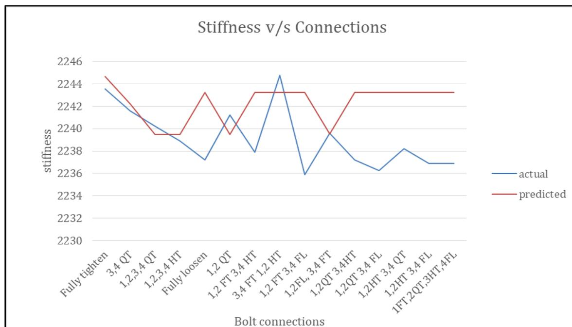
Fig 6:Stiffness vs Bolt connections
