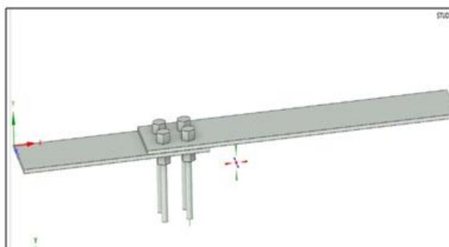
Figure 2: Geometry of the Beam modelled in ANSYS
