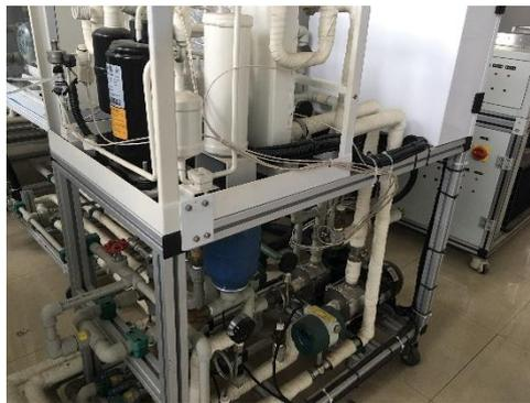
Figure 1: Modular air-conditioning system experimental device
