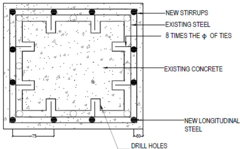
**Fig. 7: New column ties with bar anchors in case of number of new bars is more than 12 numbers**
