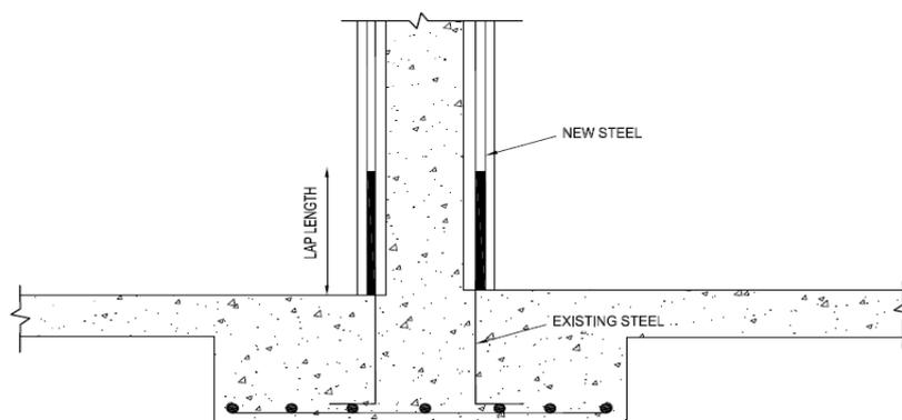
**Fig. 4: Tying of the extra steel to the existing rods for a length of lap length**
