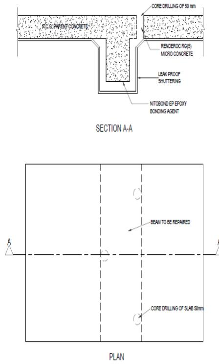
**Fig: 12 Scheme for pouring of Micro-concrete for strengthening of Beams.**
