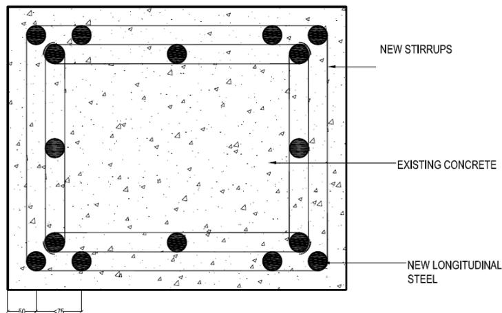
**Fig. 6: New column ties in case of number of new bars are less than 12 numbers with the spacing of the corner bar and adjacent bar less than 75mm.**
