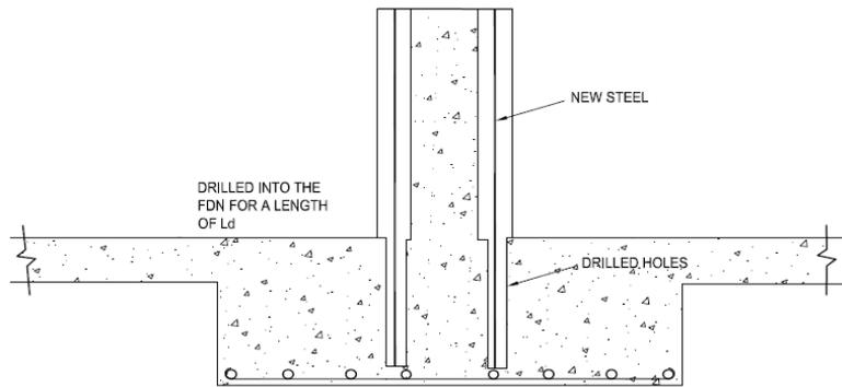
**Fig. 5: Anchoring of extra steel by drilling holes in the foundation for a length of development length in tension.**
