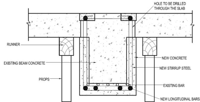
**Fig:10 Typical Strengthening of Beam and propping of slabs with a runner on sides of the beam**
