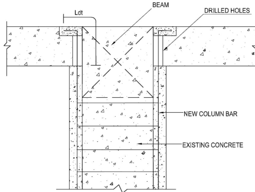
**Fig. 8: Arrangement of fixing the column bars at top- discontinuous edge.**
