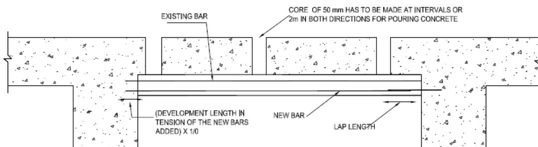
**Fig: 14 Typical Strengthening of Slab**
