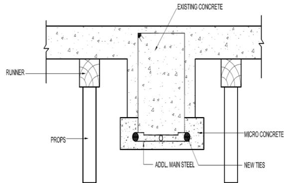
**Fig: 11 Alternative Strengthening scheme for Beam**
