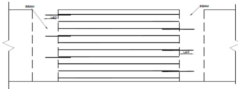
**Fig: 15 Arrangement of new reinforcement (bottom) for slab**
