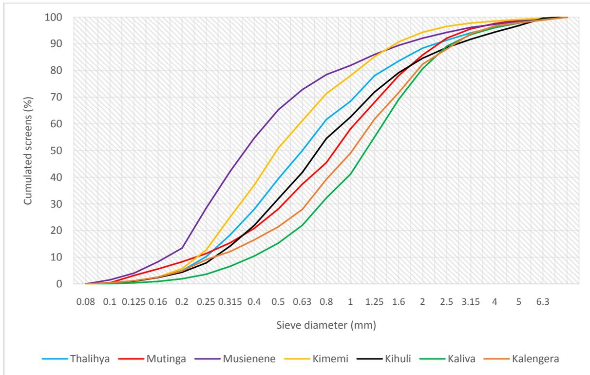
**Figure 1.** Particle size curve of Butembo sands
