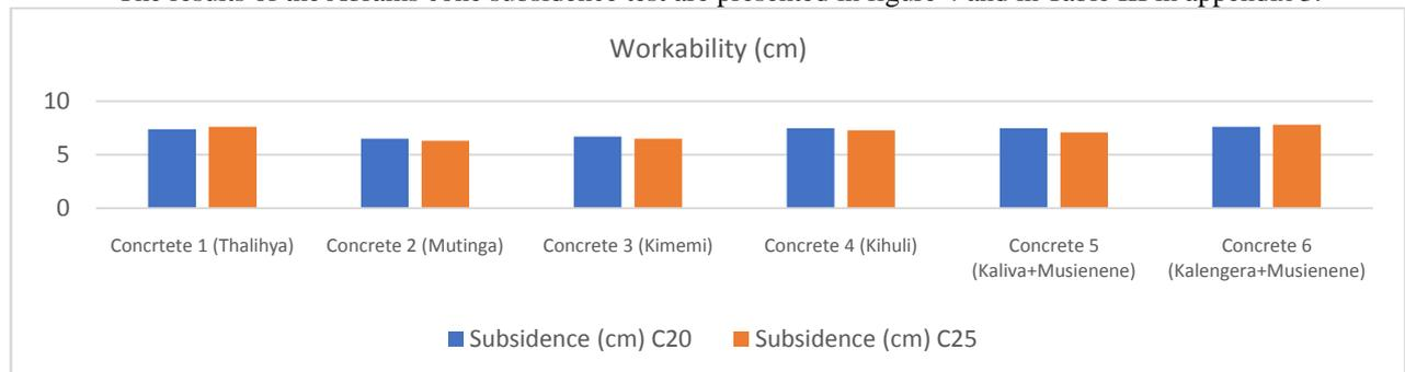
**Figure 4.** Abrams cone subsidence
