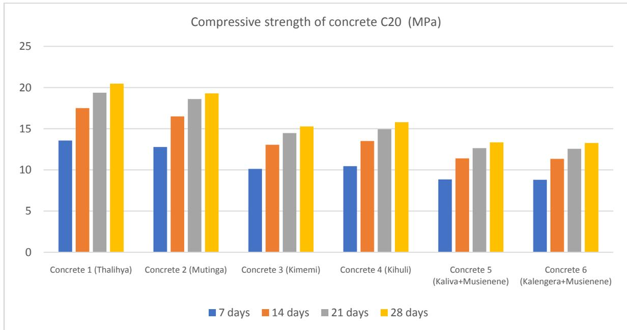
Figure 5. Concrete compression strength C20
