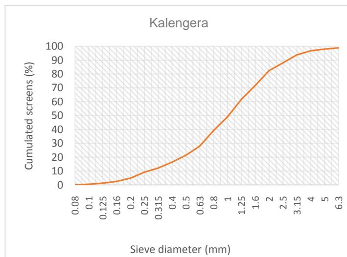
Figure g. Grain size curve of Kalengera sand
