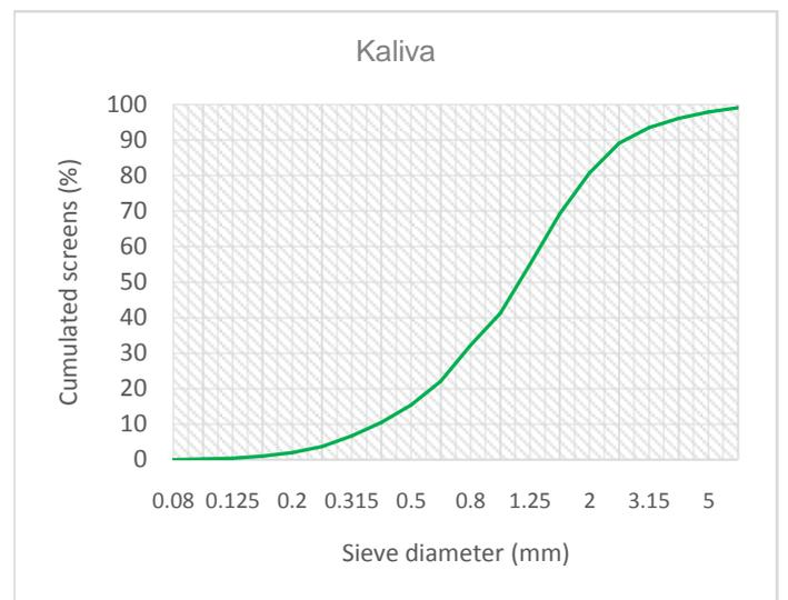
Figure f. Grain size curve of Kaliva sand
