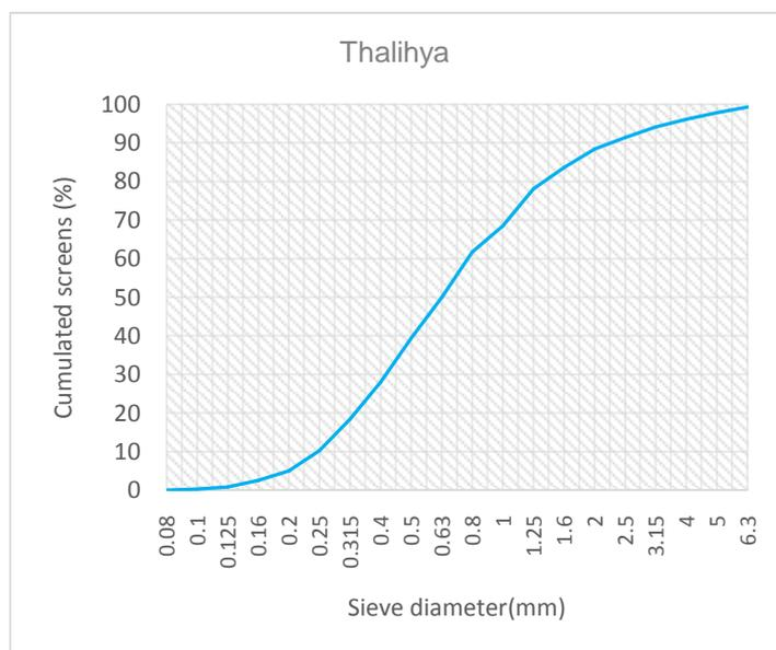
Figure a. Grain size curve of Thalihya sand
