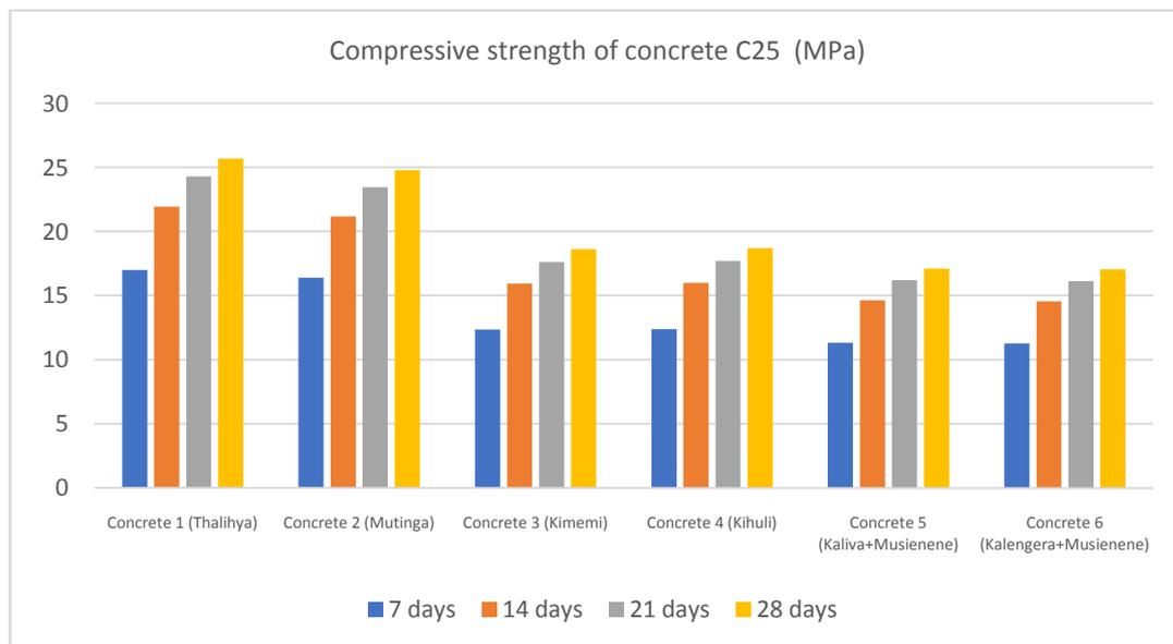
Figure 6. Concrete compression strength C25
