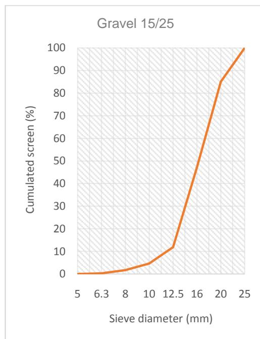
**Figure 3.** Gravel particle size curve 15/25
