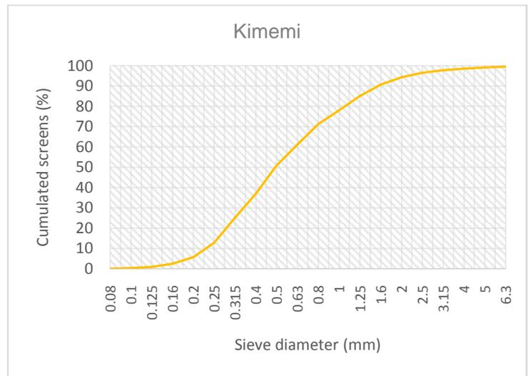
Figure d. Particle size curve of Kimemi sand
