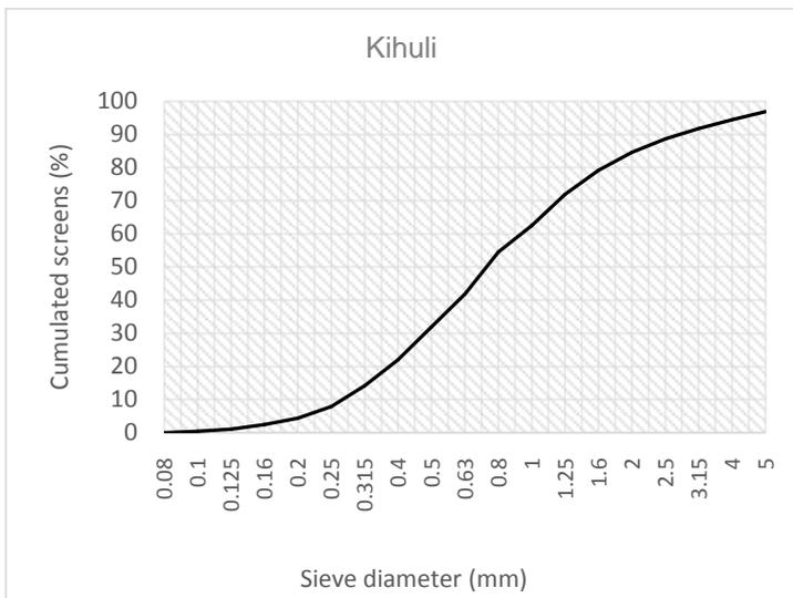
Figure e. Grain size curve of Kihuli sand
