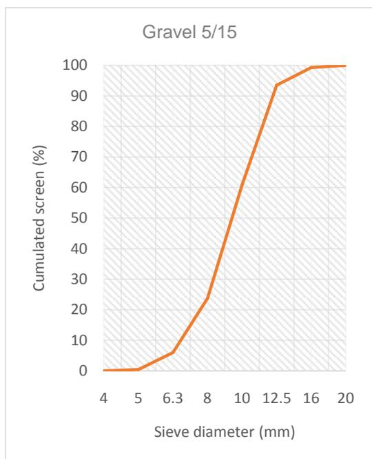
**Figure 2.** Gravel particle size curve 5/15
