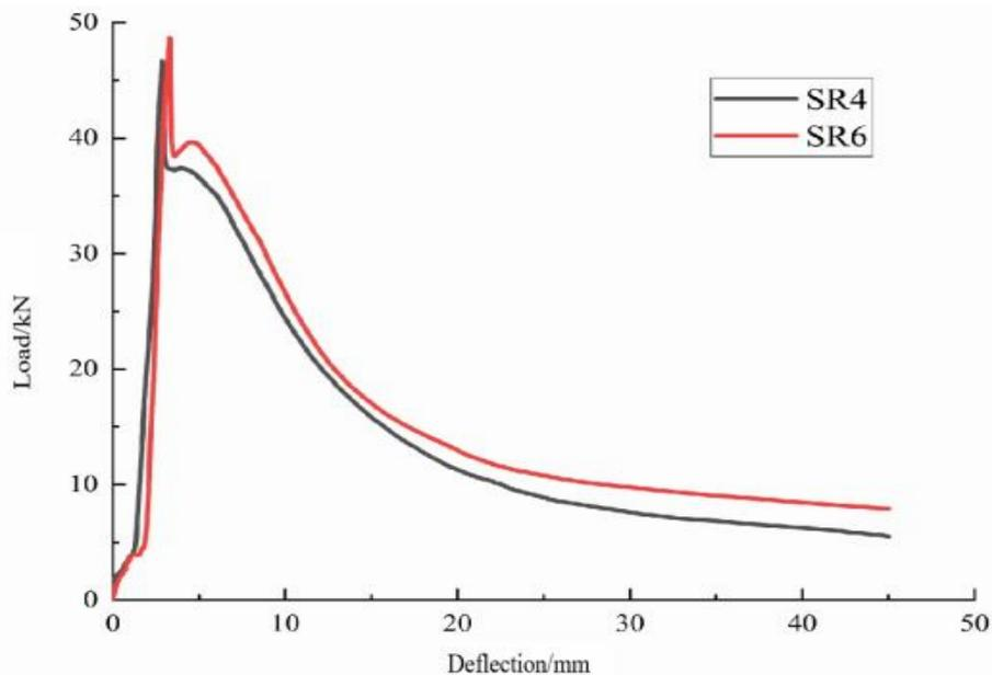
**Figure 5:** Comparison of load-deflection curves of HFRC specimens SR4 and SR6
