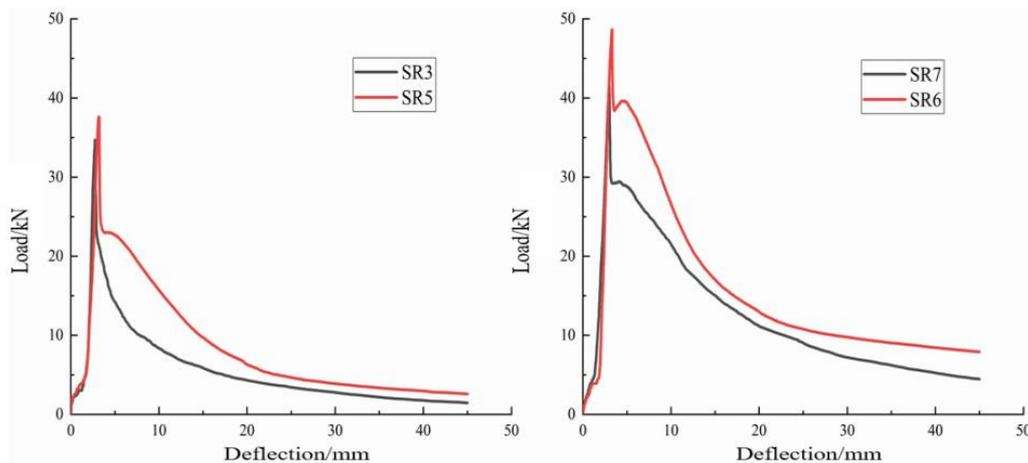
Figure 4: Comparison of load-deflection curves of HFRC specimens SR3 and SR5, SR7 and SR6
