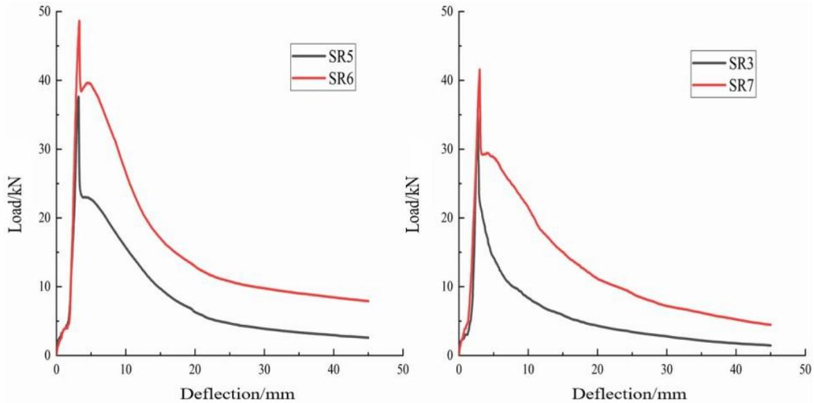
Figure 3: Comparison of load-deflection curves of HFRC specimens SR5 and SR6, SR3 and SR
