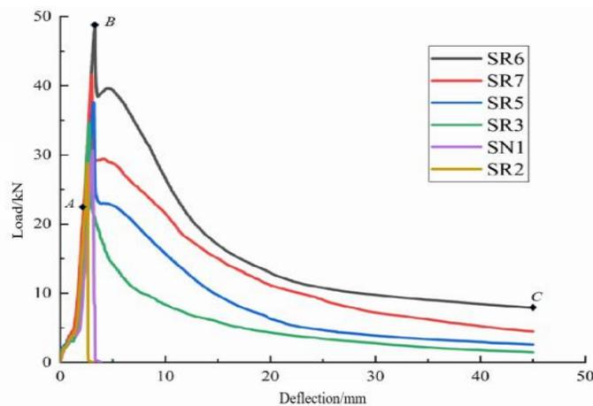
Figure 2: Load-deflection curves of recycled concrete specimens SN1, SR2, SR3, SR5~SR7
