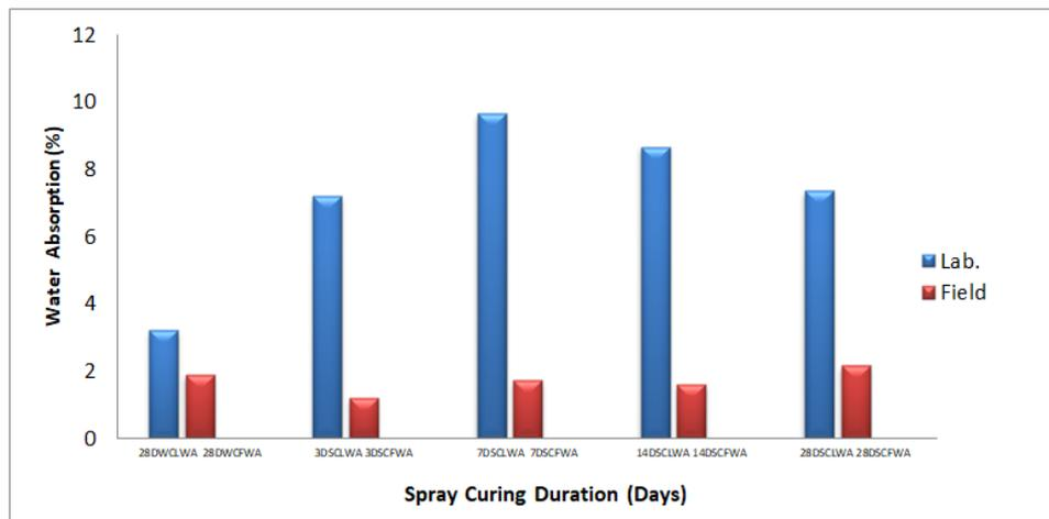
Fig. 8: Average Water Absorption at 28 Days
