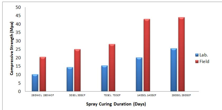
**Fig. 7: Average Compressive Strength at 28 Days**
