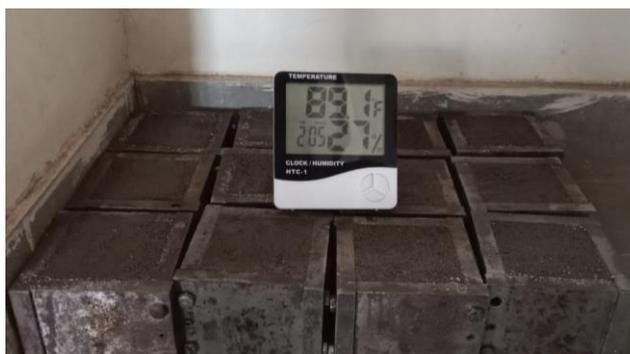
**Fig. 2: Moulds Filled with Cement-Sand Mortar**
