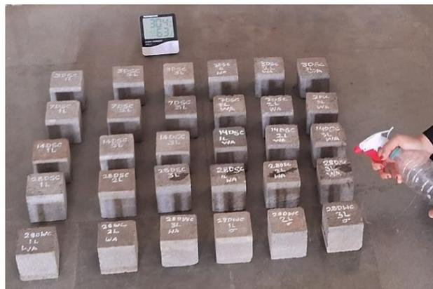
**Fig. 3: Spray Curing Being Done**
