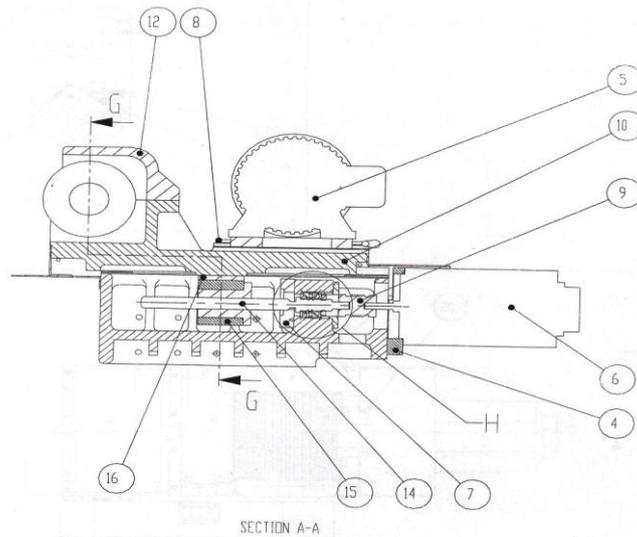
Figure1. Feed Table Sectional View
