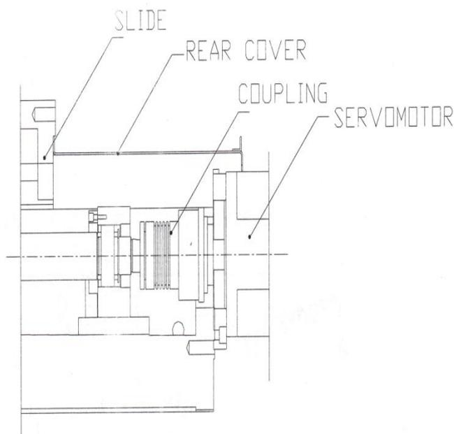
Figure6. Ball Screw Arrangement
