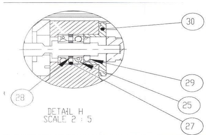
Figure2. Ball Screw Sectional View
