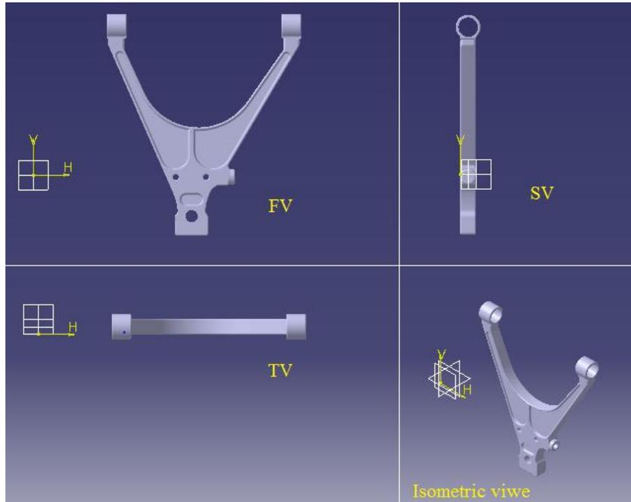
Fig. 1.1 CATIA Modeling of Lower Wishbone Arm.
