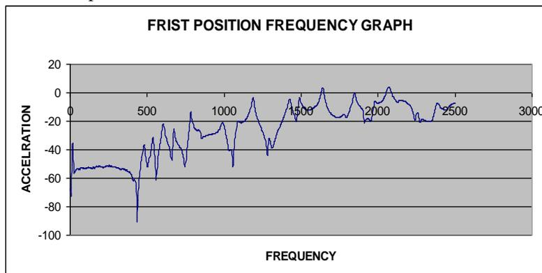
Fig.1.5 frequency graph at position near front control arm
