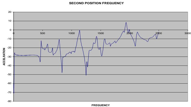
Fig.1.6 frequency graph at position near rear control arm.
