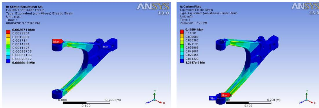
Fig. 1.3 Strain in Lower Wishbone Arm in structural steel & composite material.
