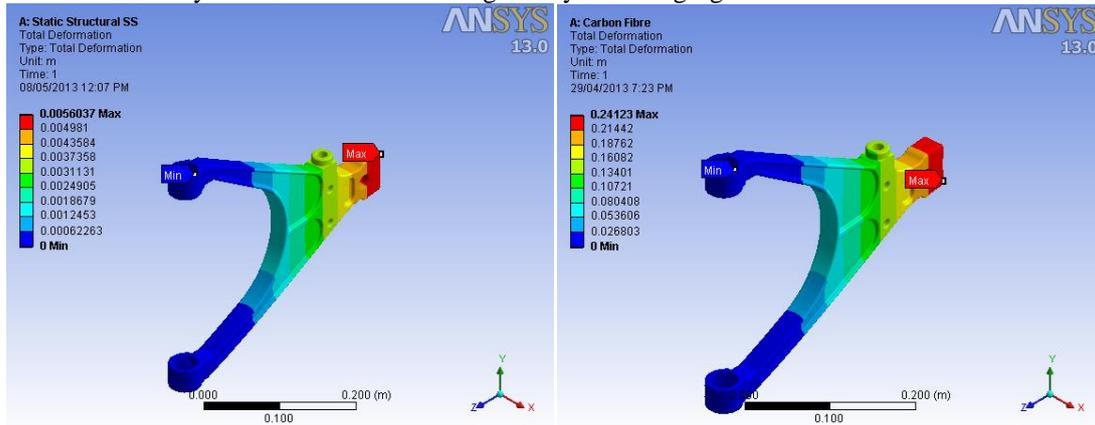
Fig. 1.4 Total deformation in Lower Wishbone Arm in structural steel & composite material.
