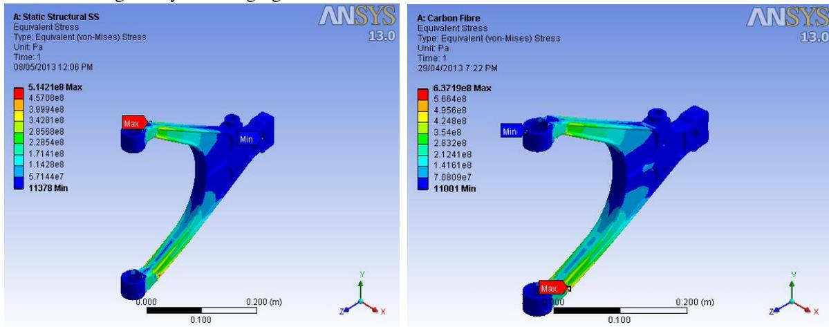
Fig. 1.2 Stress in Lower Wishbone Arm in structural steel & composite material.
