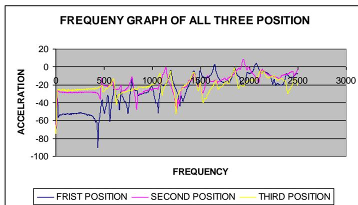
Fig.1.8 frequency graph at all three position near front control arm
