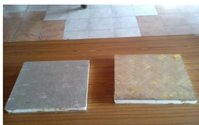
Fig.2.1: Bison Sandwich Composite (Left) Bamboo Sandwich Composite (Right)
