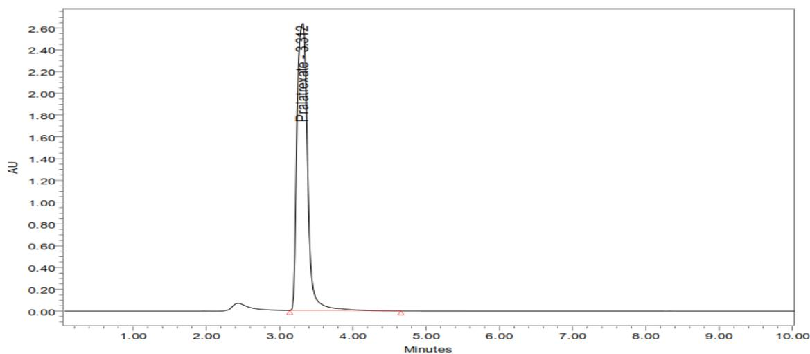
**Fig.2:** Typical RP-HPLC Chromatogram of Pralatrexate by the proposed method.
