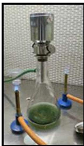
Fig. 2 - Membrane filter (Millipore filter) to obtain a cell free extract
