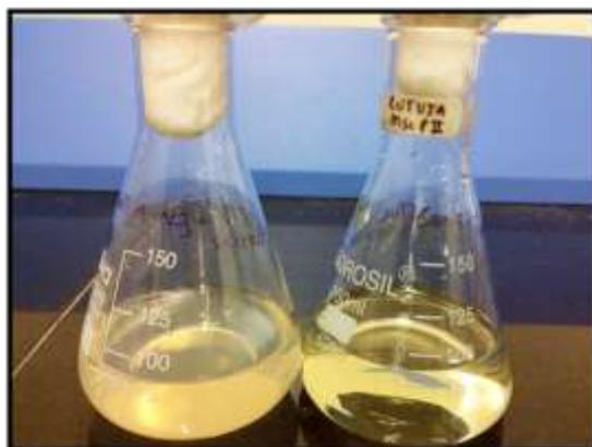
Fig. 8 - 1ml of *O. sanctum* leaves extract + 100ml OF 1mM AgNO<sub>3</sub> and CuSO<sub>4</sub> for synthesis of NPs
