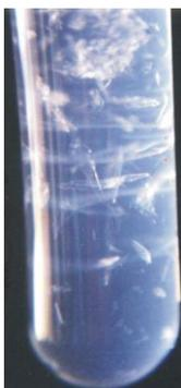
**Figure 1:** Brushite Crystals grown in gel media
