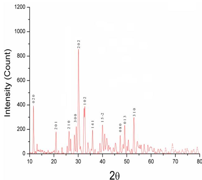
**Figure 3:** XRD pattern of brushite crystals
