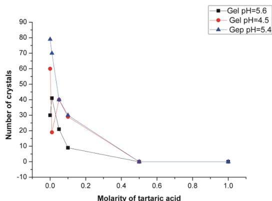
**Figure 8:** The number of brushite crystals grown Vs. the molar concentration of tartaric acid for different pH values
