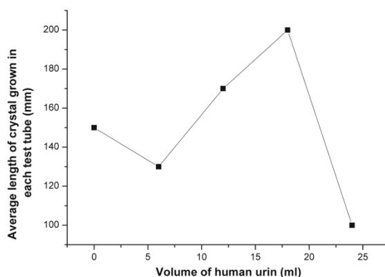
**Figure 6:** The plot of average length of grown brushite crystals Vs. volume of human urine.
