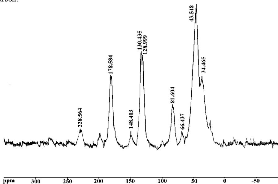
$^{13}\text{C}$ / NMR of PS-NVP-HDODA polymer support
