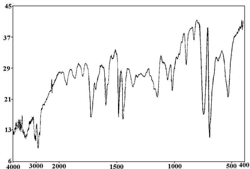
**IR (KBr) spectrum of PS-NVP-HDODA polymer support**
