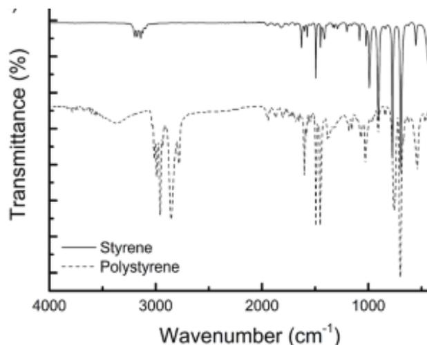
Fig. 3. Example of FTIR Spectrum from Polystyrene and Styrene<sup>16</sup>
