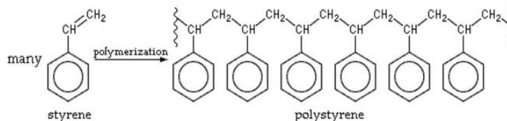
Fig. 1. The Chemical Formula of Polystyrene<sup>8</sup>
