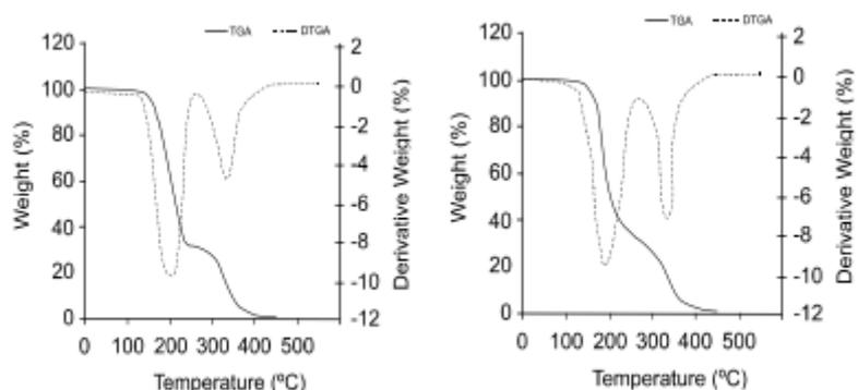
**Fig. 11. TGA Thermogram of PS - Starch Blend<sup>31</sup>**
