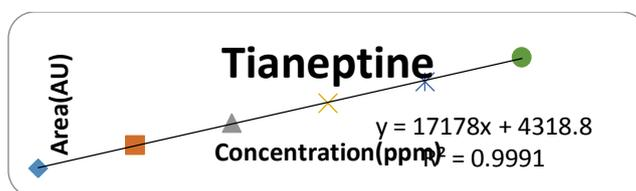
**Precision:** Obtained Five (5) replicates of 100% accuracy solution as per experimental conditions. Recorded the peak areas and calculated % RSD.
