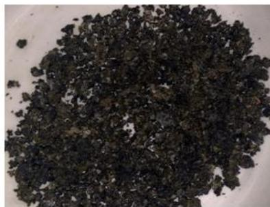
Figure 4. Dry extracted pectin pellets.
