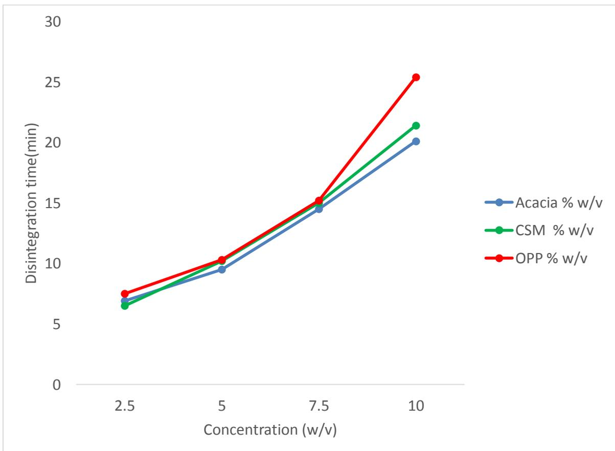
Figure 7. Relationship of binder concentration versus disintegration time of erythromycin tablet
