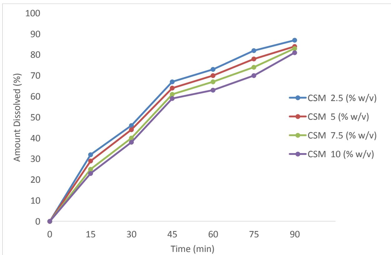
Figure 9. Dissolution profile of erythromycin tablet formulated with varying conc. of corn starch mucilage (CSM).
