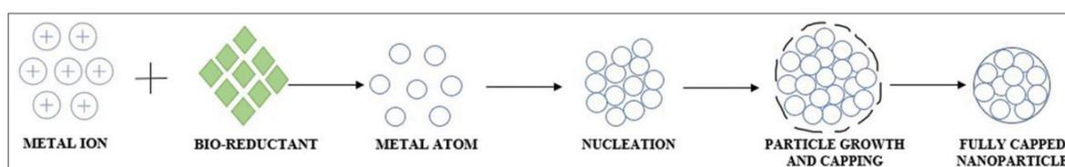
Figure 2. Microbial synthesis of nanoparticle
