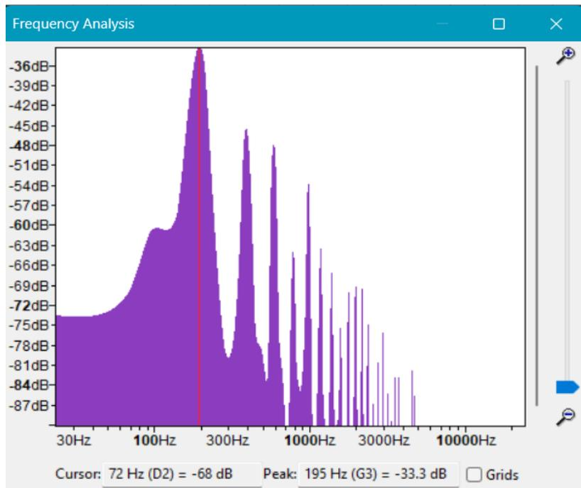
Fig.5 Frequency spectrum of open G string plucked by plectrum
