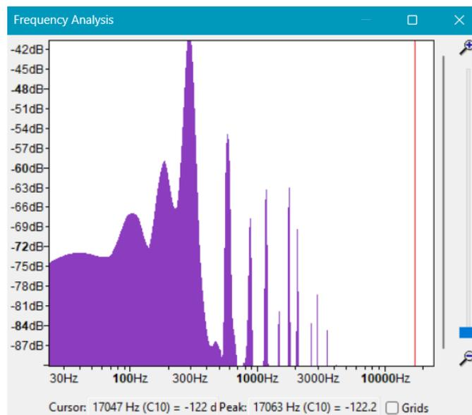
**Fig.12 Frequency Spectrum of the natural harmonic produced on the 7<sup>th</sup> fret**
