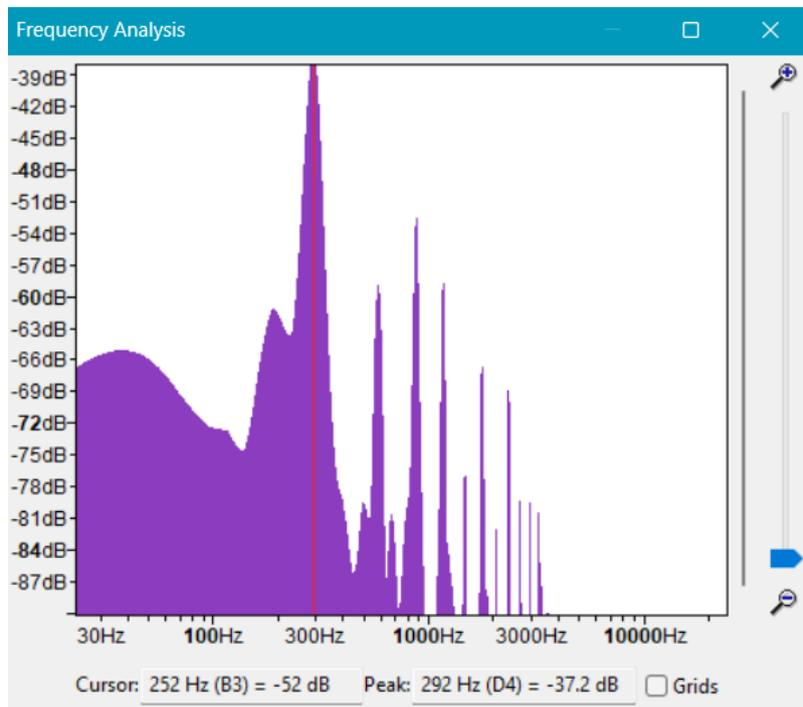
Fig.13 Frequency Spectrum of the artificial harmonic of the 7<sup>th</sup> fret
