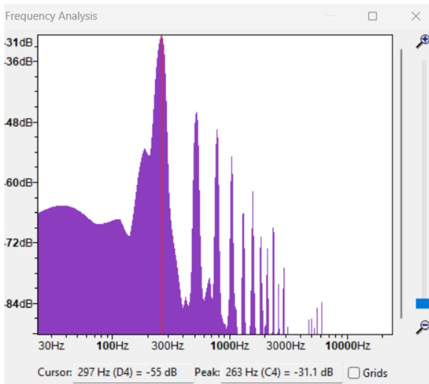
**Fig.11 Frequency Spectrum of the artificial harmonic of the 5<sup>th</sup> fret**
