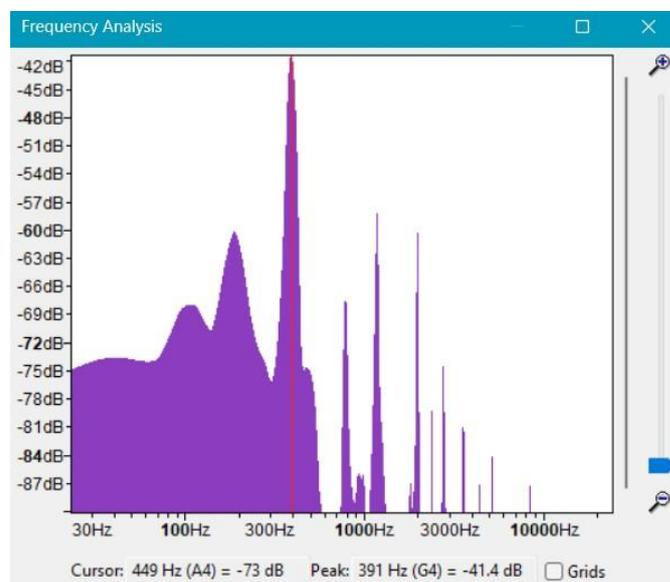
Fig.8 Frequency Spectrum of the natural harmonic produced on the 12<sup>th</sup> fret
