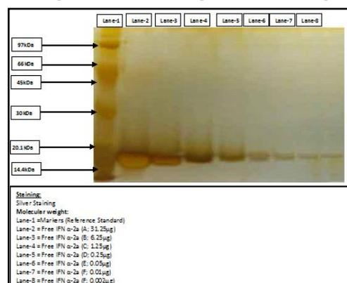
Silver staining detected IFN  $\alpha$ -2a up to 0.002 $\mu$ g i.e. 25% more sensitive than coomassie staining as shown from lane-8, as very clear band is observed. Thus this technique is suitable for impurities estimation up to 0.002 $\mu$ g.
