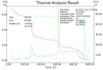
Fig. 6: Thermogravimetric analysis of nanocomposite.
