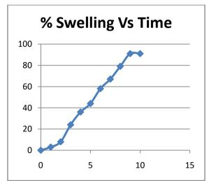
Figure 7. Water Absorption of the chitosan-sodium alginate nanocomposites
