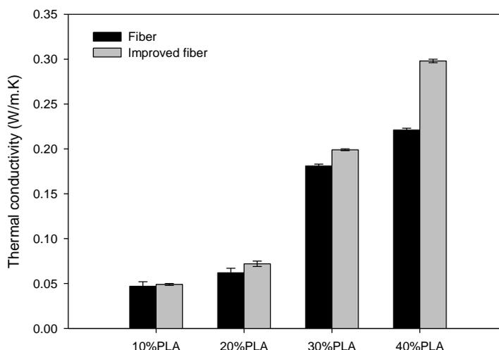
**Fig.8 The Thermal conductivity of composite prepared from PLA/fiber and PLA/improved fiber**
