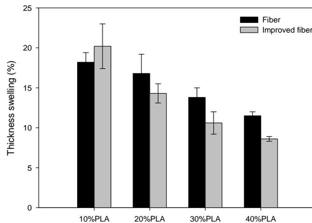
**Fig.5 The thickness swelling of composite prepared from PLA/fiber and PLA/improved fiber**
