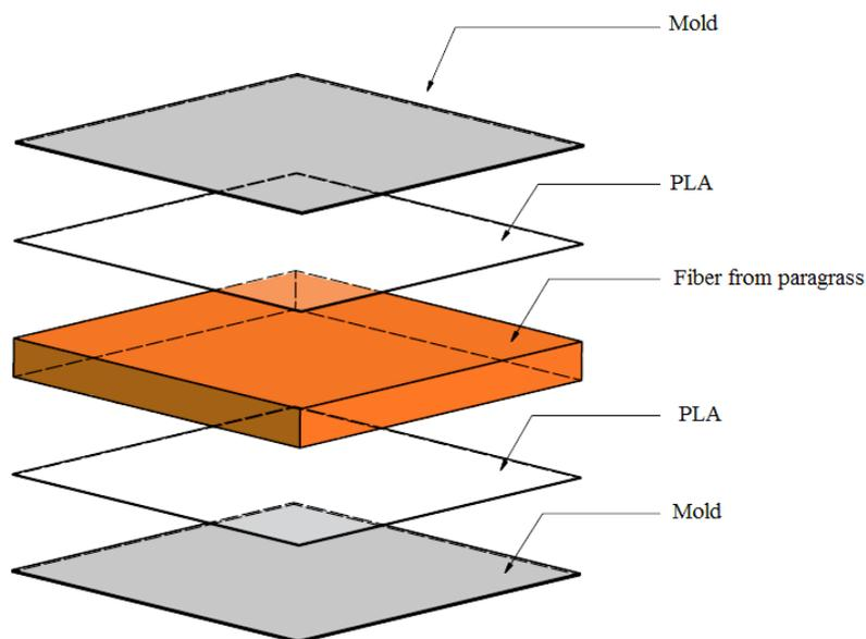
**Fig. 1 Preparation of composite from PLA and paragrass fiber by laminated technique**
