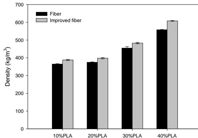
**Fig. 3** The density of composite prepared from PLA/fiber and PLA/improved fiber
