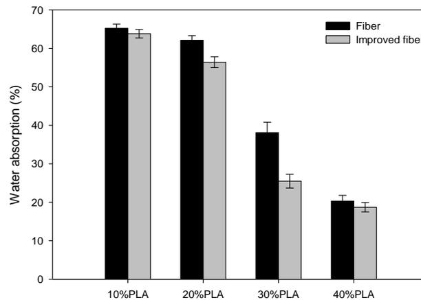
**Fig. 4** The water absorption of composite prepared from PLA/fiber and PLA/improved fiber
