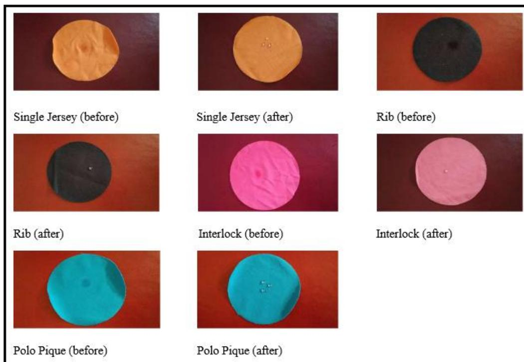
**Figure 1:** Drop test on treated fabrics and their visual appearance
