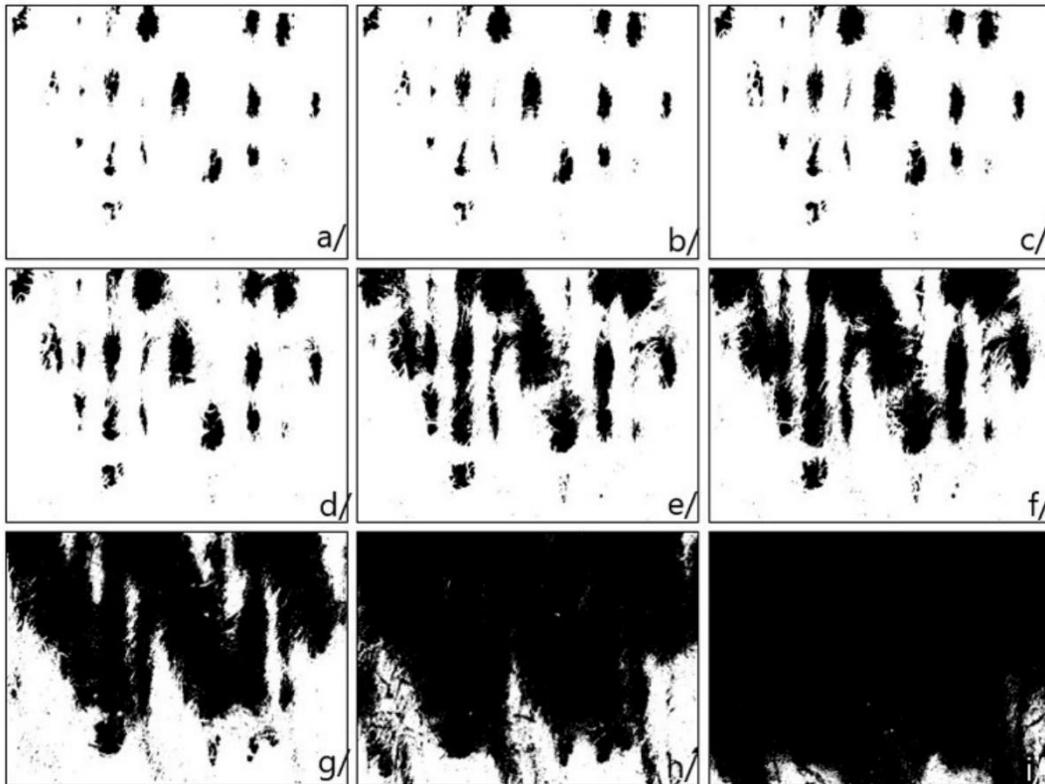
**Figure 3:** Image segmentation of Sample 5, using different threshold levels T: a/ T=40, b/ T=60, c/ T=80, d/ T=100, e/ T=120, f/ T=140, g/ T=160, h/ T=180, i/ T=200.
