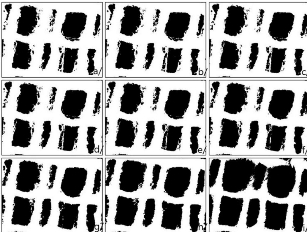
Figure 2: Image segmentation of Sample 1, using different threshold levels T: a/ T=40, b/ T=60, c/ T=80, d/ T=100, e/ T=120, f/ T=140, g/ T=160, h/ T=180, i/ T=200.
