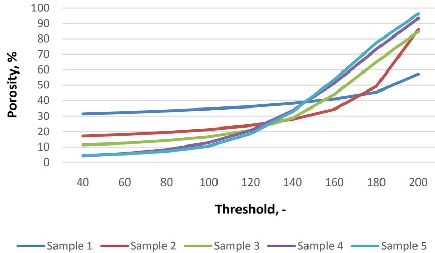
**Figure 4:** Porosity change as a function of the image segmentation threshold
