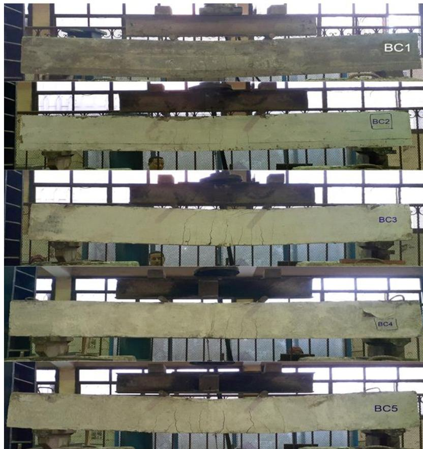
Fig. 26: Cracking Pattern and Mode of Failure for control beam (BC)
