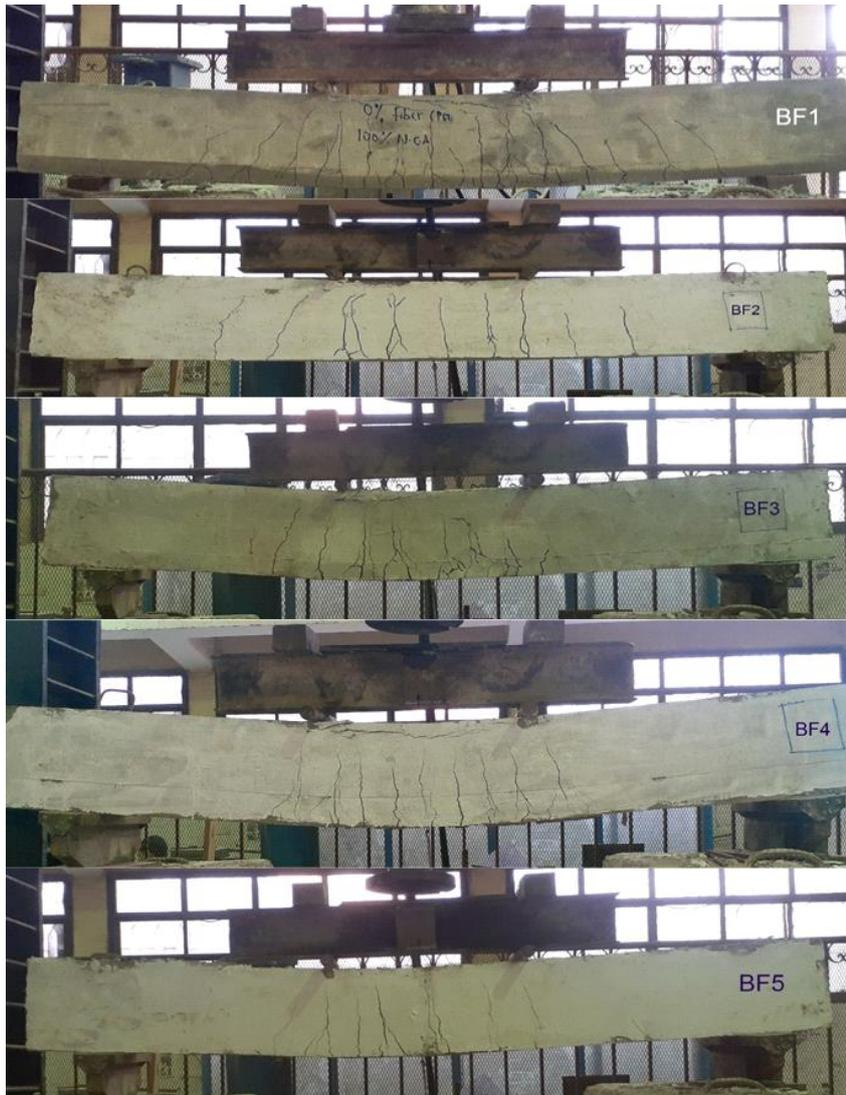
**Fig. 27:** Cracking Pattern and Mode of Failure for weak in flexure beam (BF)
