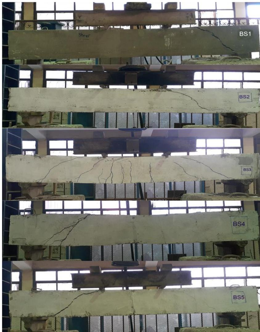
**Fig. 28:** Cracking Pattern and Mode of Failure weak in shear beams (Bs)
