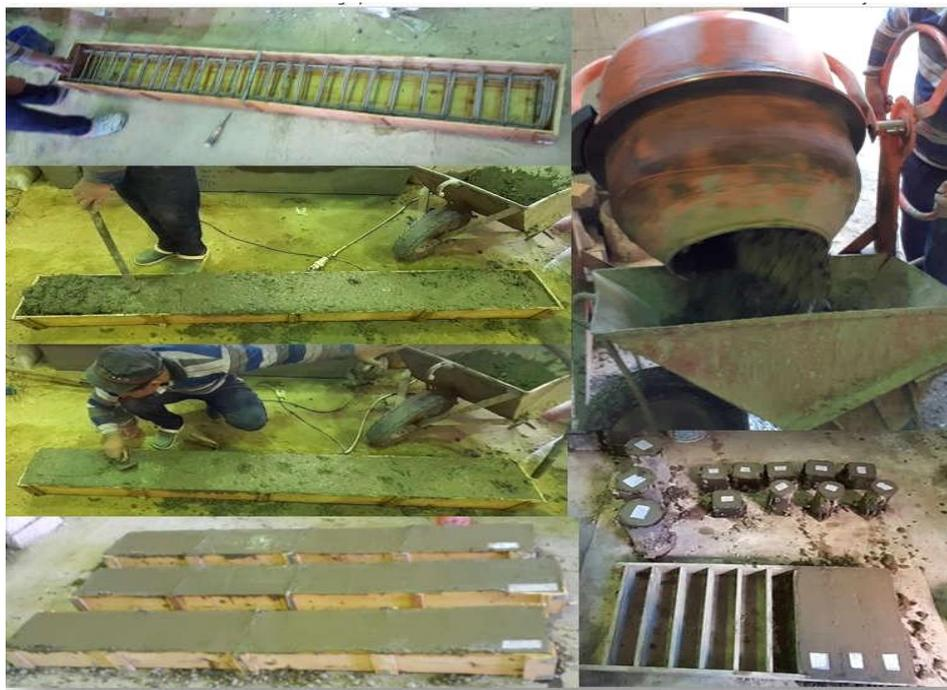
Fig. 9: Preparation of test specimens (Cubic, Cylinders and Beams)
