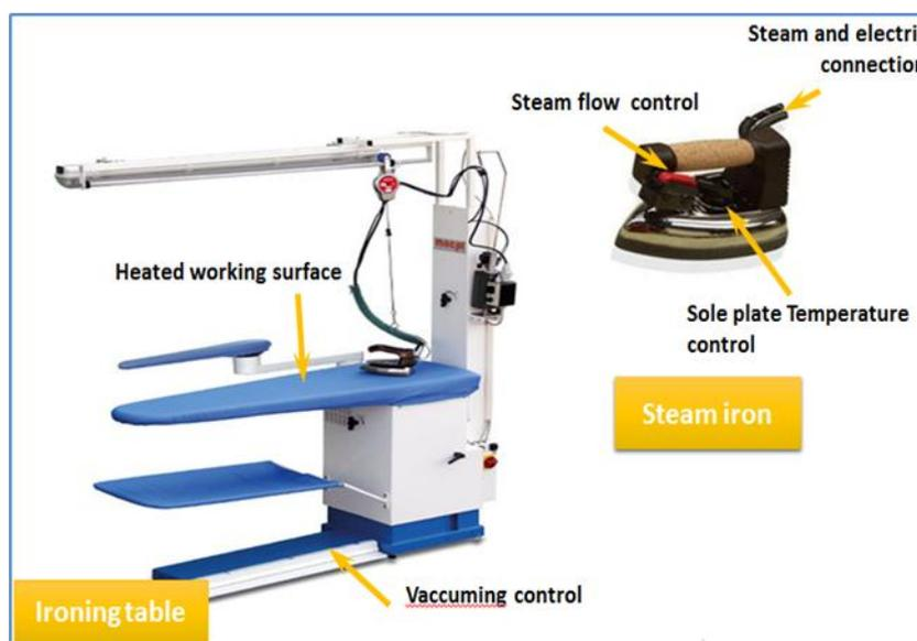
Figure no 2: Ironing apparatus
